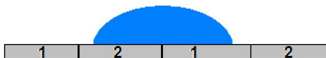
Figure 4-3: Representation of a chemically heterogeneous surface where 1 and 2 represent different surface chemistries.
