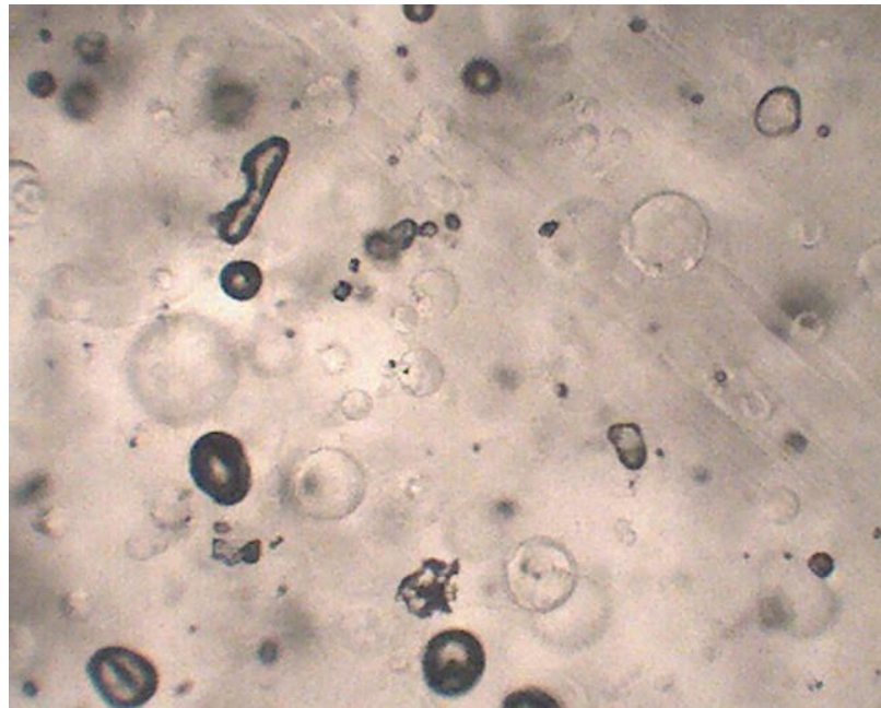
Figure 7: The distribution of micro-capsules in a self-healing specimen using MeMal-4MeOSt-DVB healing agents viewed by optical microscopy (magnification of 20×)
