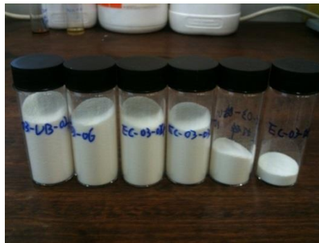
Figure 4.1: Micro-capsules containing different healing agents
