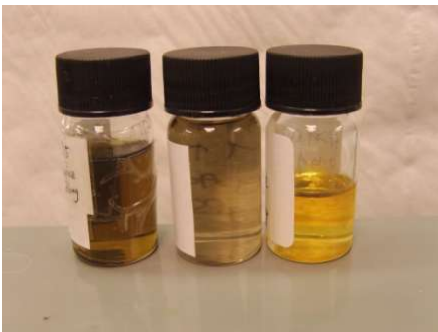
Figure 35: Photograph of the waste residues post filtration in THF. left = 60 minutes, middle = 30 minutes, right = virgin polystyrene 60 minutes.
