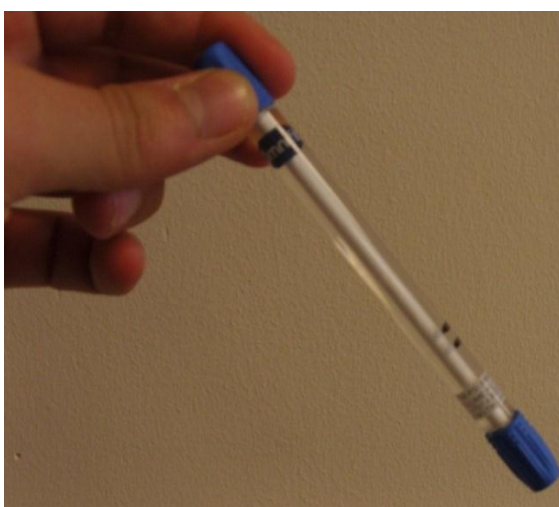
Figure 2:6 – Photopolymerised GMA-based polyHIPE monolith covalently bound to a functionalized glass chromatography column
