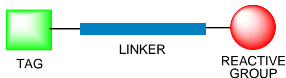
Figure 1.17 Cartoon representation of the general structure of a reactivity probe, which contains a reactive group, linker and tag.
