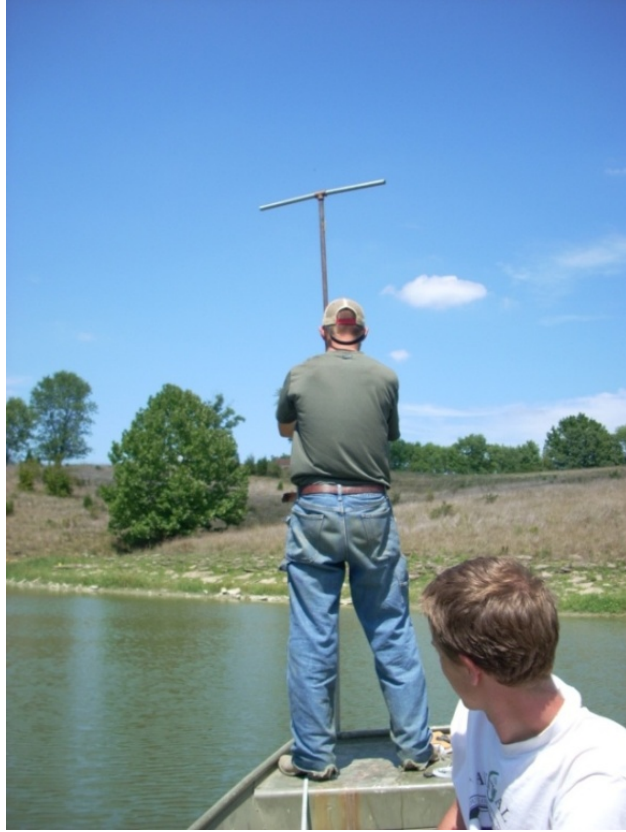
FIGURE 19 - Taking a core, note operator standing on steel tape to position corer along cross section
