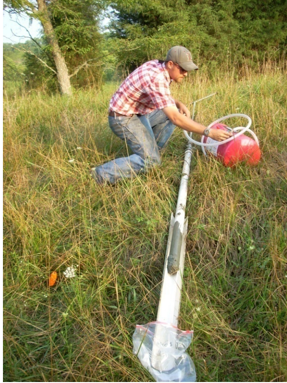
FIGURE 21 - Operator prepares to extract core into cradle; note bag to collect core water
