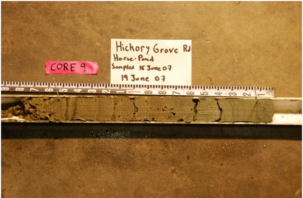
FIGURE 23 - Photo of split pond core exhibiting the three sediment zones and internal structures
