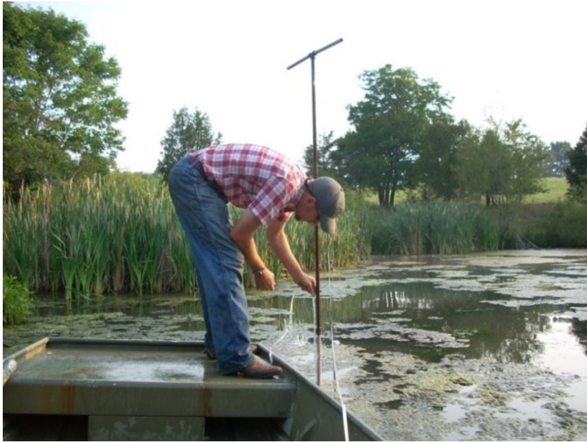
FIGURE 17 - Taking sediment depth measurements as part of the bathymetric survey, note steel tape used to position sediment probe
