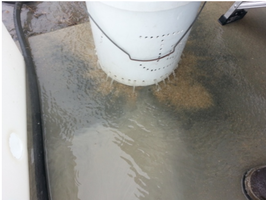
Figure 16: Washing the aggregate using a pressure washer
