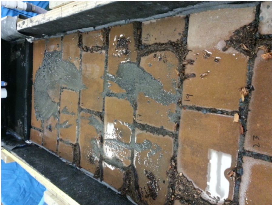
Figure 35: Experiment #4, 1% slope, 6 mm gap size, no aggregate between the pavers
