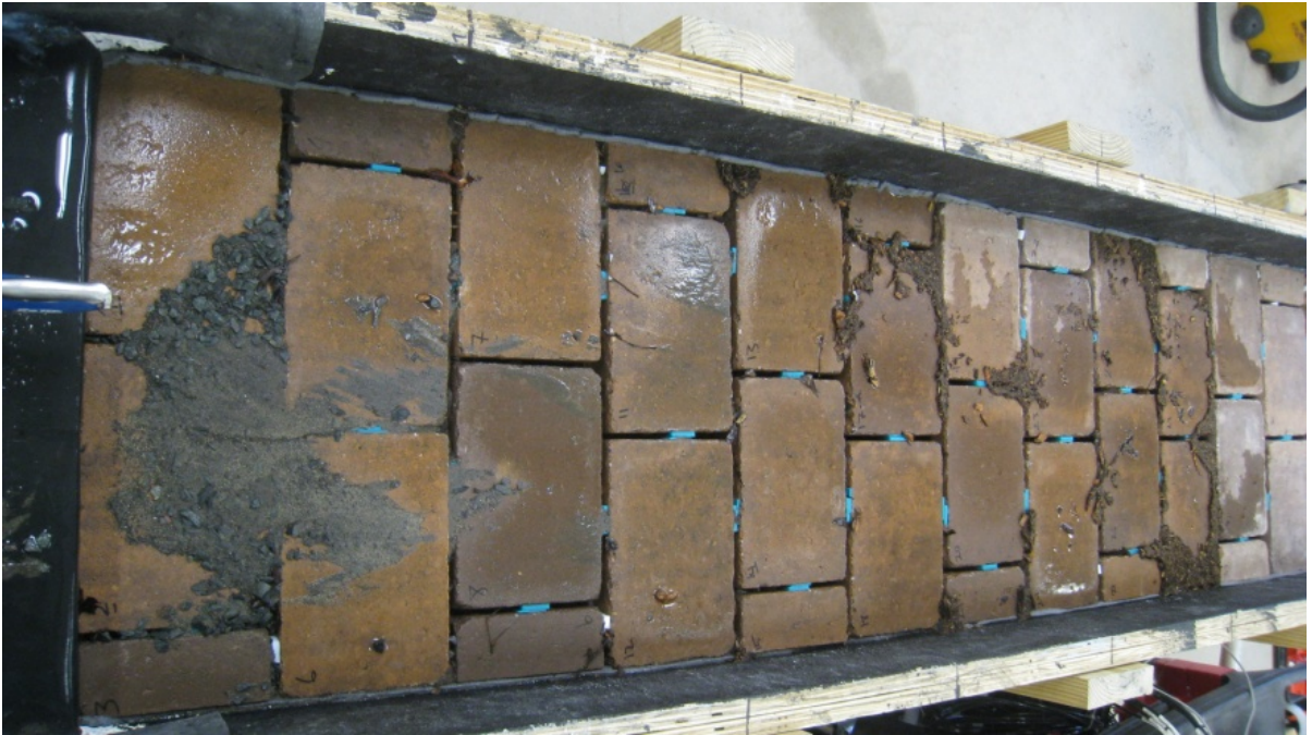
Figure 32: Experiment #1, 1% slope, 6 mm gap size, no aggregate between the pavers
