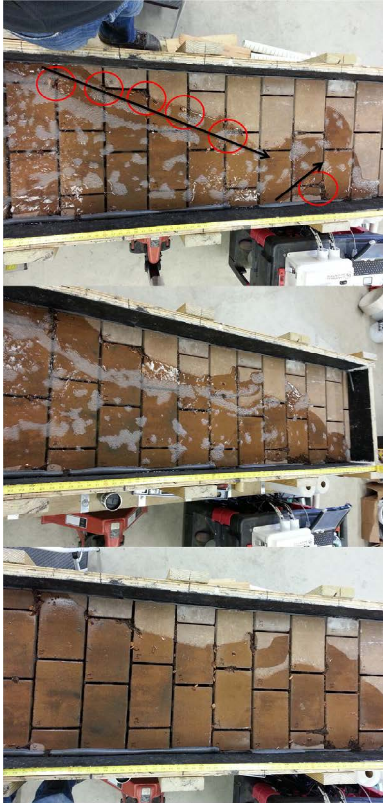
Figure 38: Stormwater runoff flow unpredicted pattern in experiment #5
