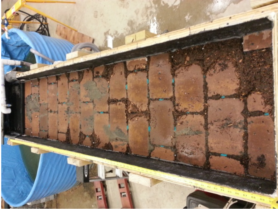
Figure 35: Experiment #4, 1% slope, 6 mm gap size, no aggregate between the pavers
