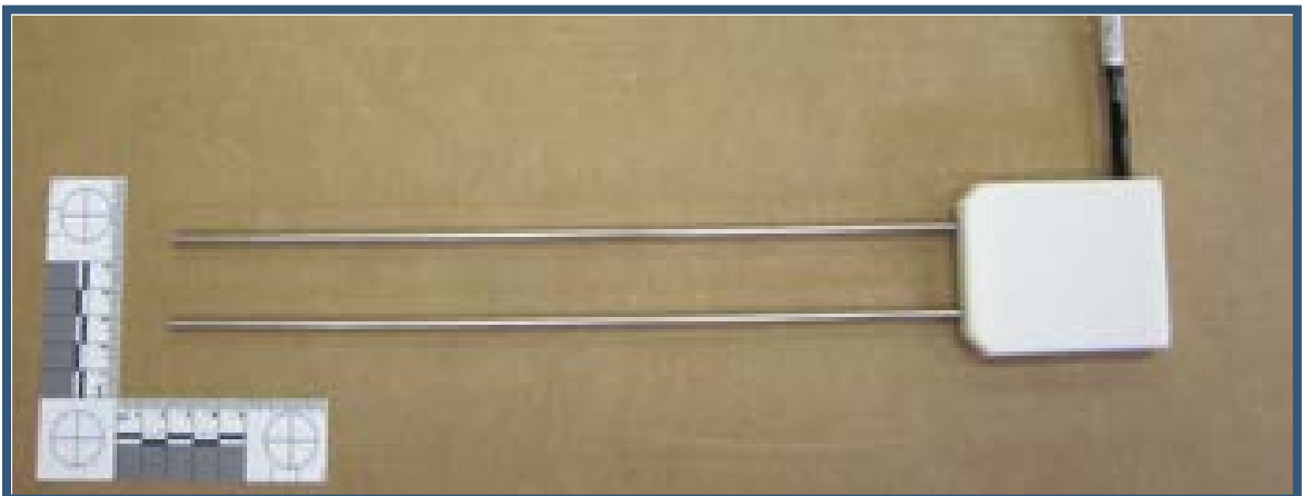
Figure 20: Time domain reflectometer (TDR)
