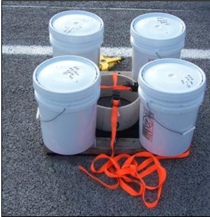
Figure 22 - Surface Infiltration Test Apparatus (Borst et al. 2010)
