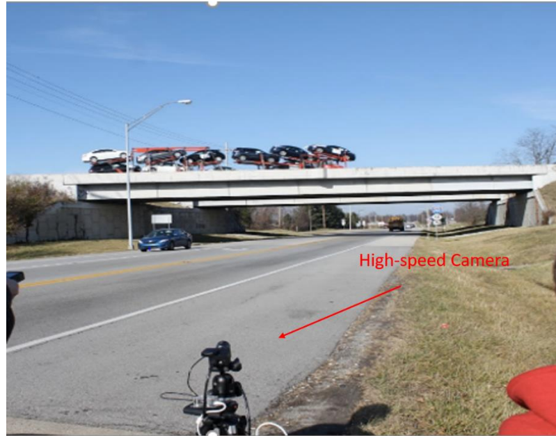
Figure 2.5. Application of High-speed Camera on Highway Bridge Vibration
