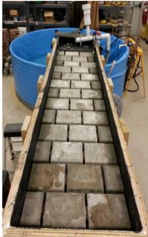
Figure 17. Flume's paved surface (a) Coventry I (b) Eco-Cobble (c) Eco-Paver
