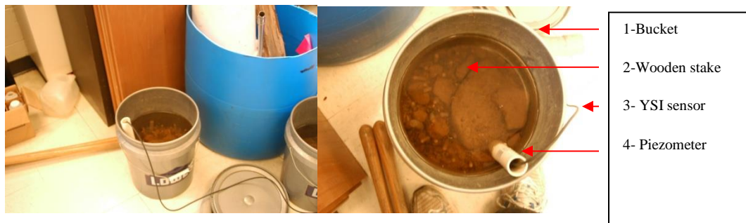
Illustration 7.4. Bucket with piezometer and wooden stake inside.
