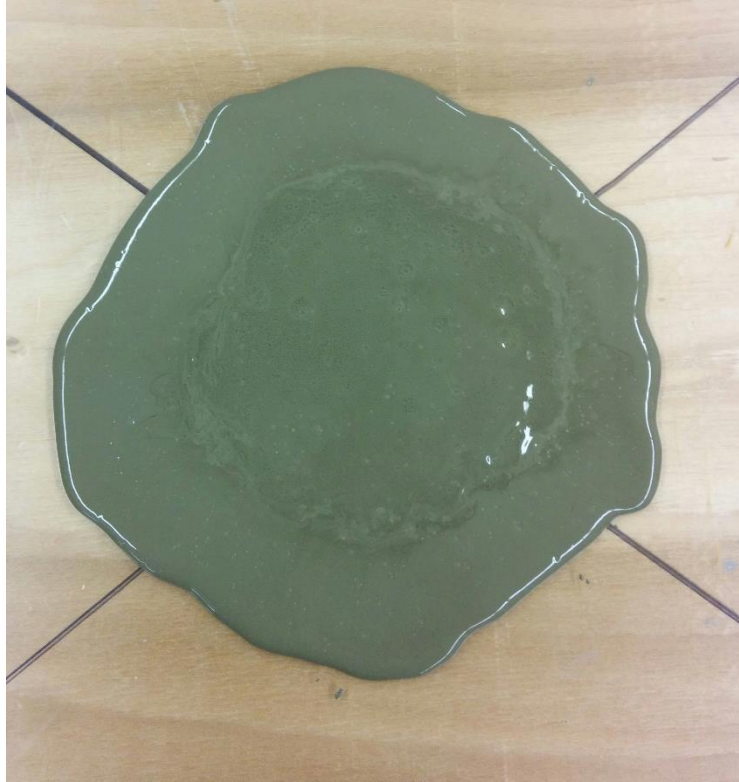
FIGURE 29 – SLUMP DIAMETER TEST P55-0-0
