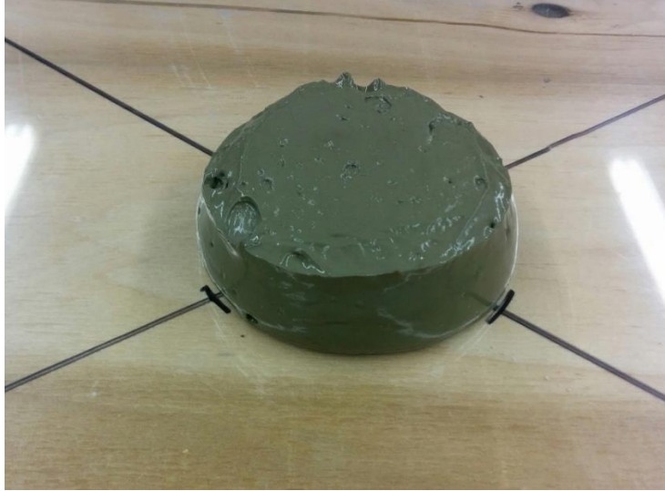
FIGURE 27 – SLUMP DIAMETER TEST P35-0-0
