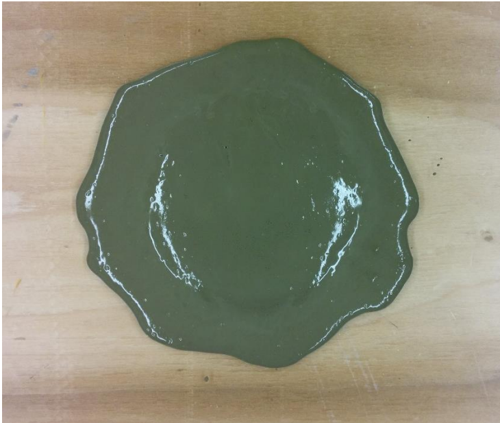
FIGURE 28 – SLUMP DIAMETER TEST P45-0-0
