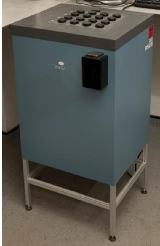
FIGURE 18 – TAM AIR CALORIMETER (Black)
