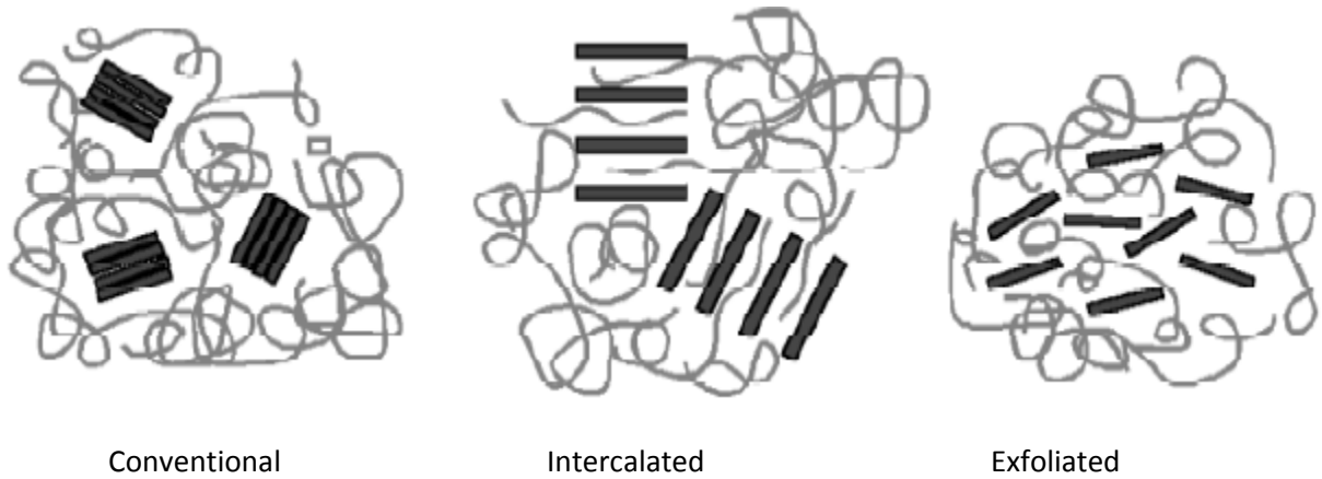
Figure 1-9. Different microstructure morphology of organoclays (Giannelis et al. 1999)
