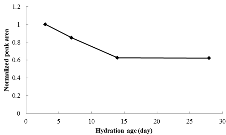
Fig. 5.6. Evolution of peak area for calcium silicates in the ordinary paste at the hydration ages from 3 to 28 days
