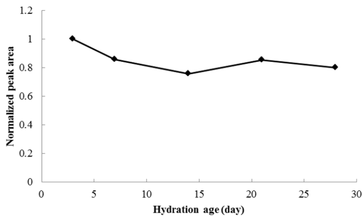
Fig. 5.9. Evolution of peak area for silica fume in UHPC at the hydration ages from 3 to
