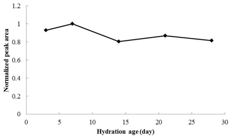
Fig. 5.10. Evolution of peak area for calcium silicates in UHPC
