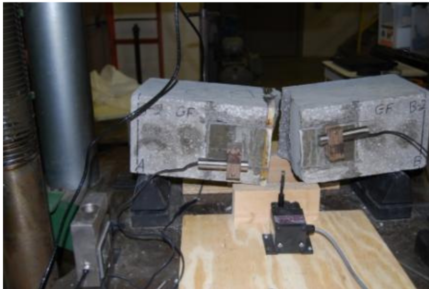
FIGURE 50. Typical Glass Fiber Rupture Failure
