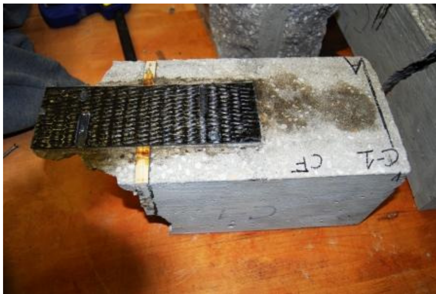
FIGURE 46. Carbon Interfacial Shear Debond (Specimen C-1, a 100% Bond Area Specimen) with the Largest Amount of Fractured Concrete Material
