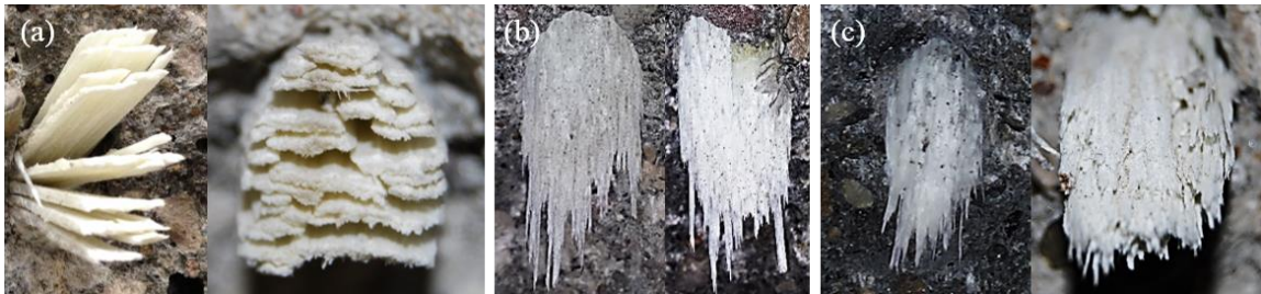
FIGURE 21 – Failure Modes: (a) Mode I, 45°; (b) Mode II, 135°; (c) Mixed Mode, 90°
