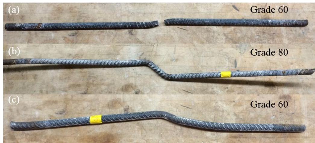
FIGURE 22 – Steel Failure and Deformation: (a) 135°; (b) 45°; (c) 90°
