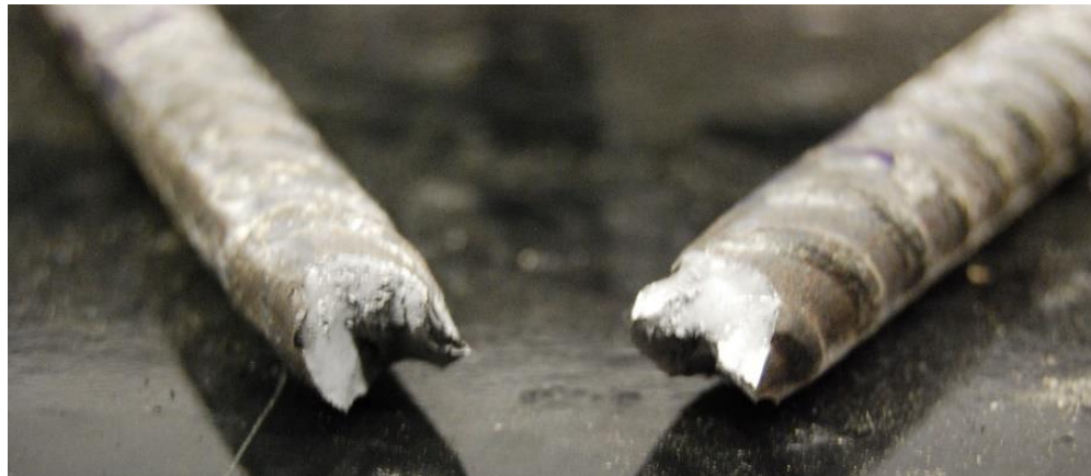
FIGURE 19 – Failure of Steel Tension Specimen
