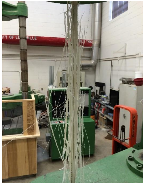
FIGURE 17 – Failure of GFRP Tension Specimen
