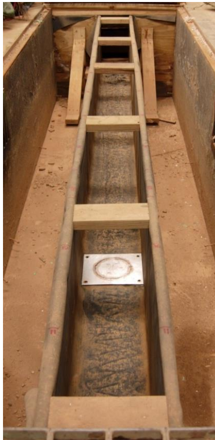
Figure 8. Multi-channel PBIS installed on the flume bed 2.67 m downstream from sediment-feeding location
