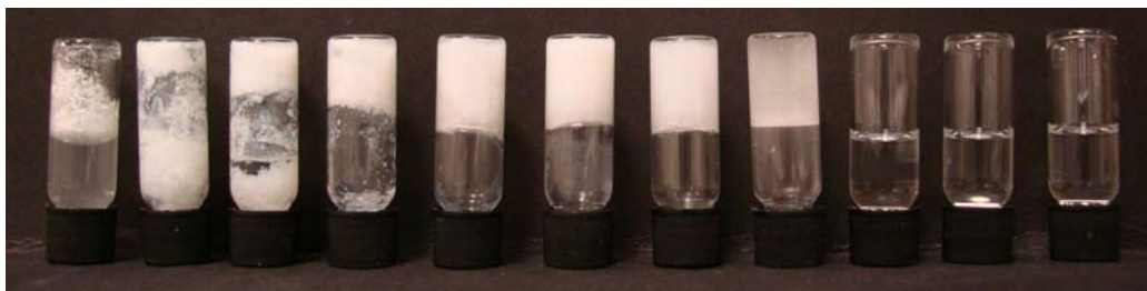
Figure 2.2. DMSO:Water gels formed by the addition of water to a solution of 2.1a in DMSO. From left to right the solvents are: pure water, ratios 1:9; 2:8; 3:7; 4:6; 5:5; 6:4; 7:3; 8:2; 9:1; pure DMSO. Note that the more aqueous samples, 1:9; 2:8; 3:7, are precipitated and/or form weak gels. Note the 8:2; 9:1 and pure DMSO samples are clear solutions.
