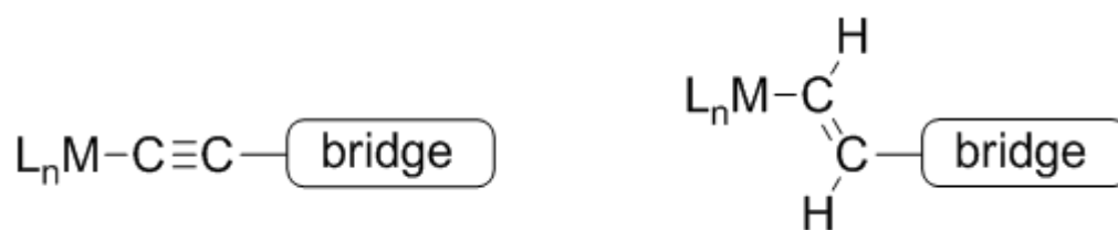
Figure 7 Representations of mono-metallic bridge complexes with an; (left) ynyl linker, and (right) enyl linker ( trans -).
