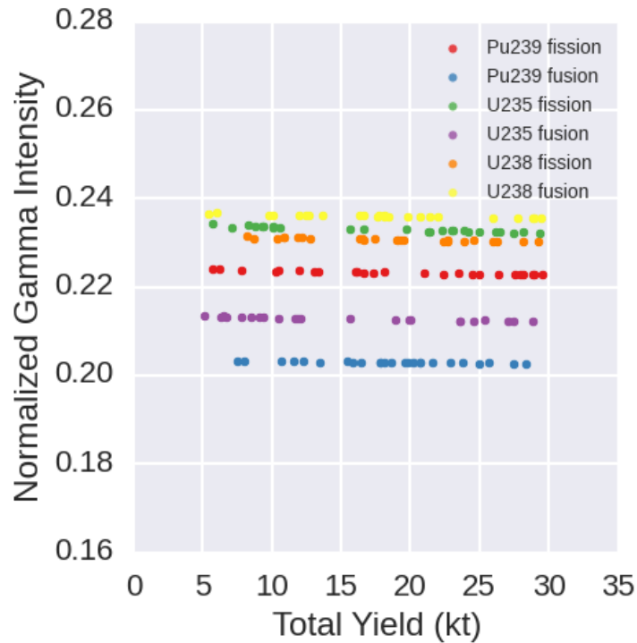
Figure 3-12 Normalized gamma intensity of the ^{99}\text{Mo} 140.5 keV line while varying both burst height and total yield
