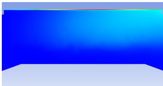
Figure 47: RT-4 window hotspot temperature distribution close-up
