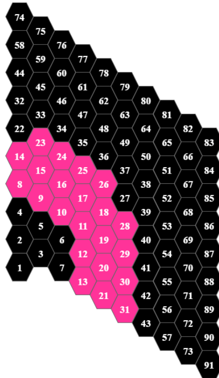
Figure 31. MHTGR-350 one-third core model representation. Blocks 1-7 , 22, 27 and 32-91 are reflector blocks. Blocks 8-21, 23-26 and 28-31 are fuel blocks
