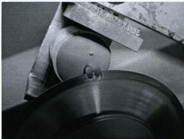
Figure 3-19 The top part of the proximal metaphysis was trimmed by the diamond saw
