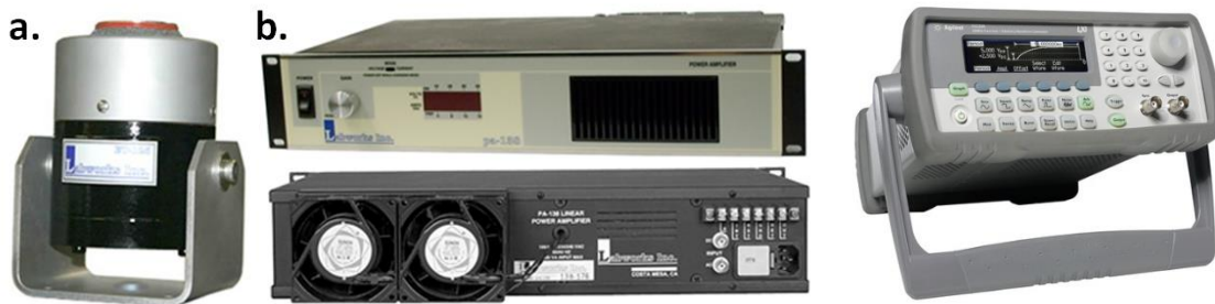
Figure 3.13. Images of a.) electrodynamic shaker, b.) linear power amplifier, and waveform generator.
