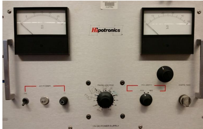
Figure 3.15. Image of front panel of the Hipotronics R30B HV DC power supply.
