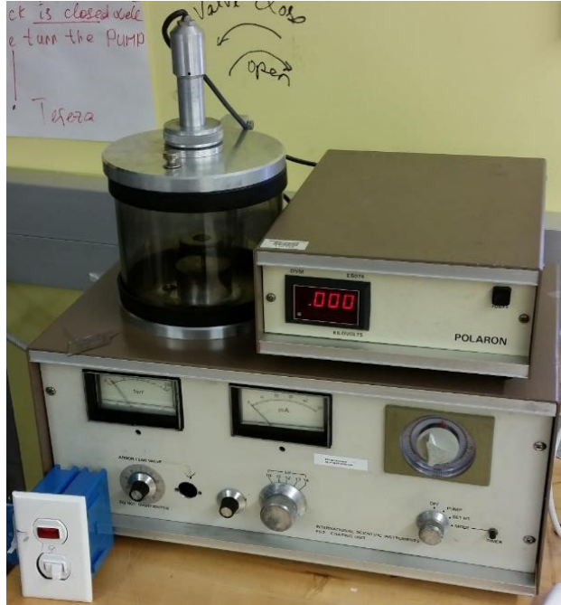
Figure 3.11. DC Sputtering System for applying gold onto SFCS substrates.
