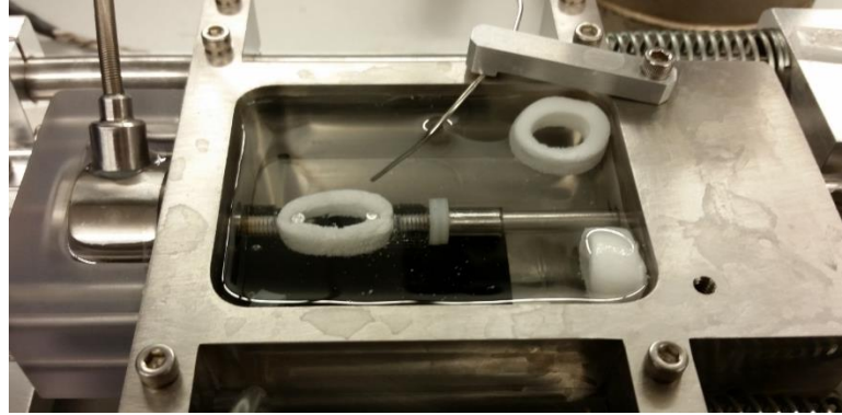
Figure 4.23. Image of SFCS-ZnO sample mounted in custom ring testing fixture
