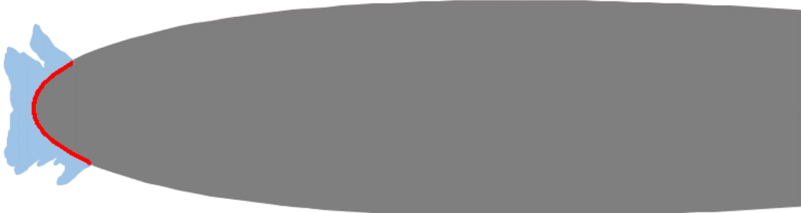
Figure 43. Illustration of A and W variables. A is the cross-sectional area of the ice (light blue area), and W is the length of the red line. Gray area is a cropped NACA 0012 airfoil.
