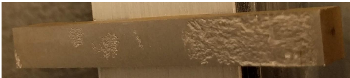
Figure 81. Surface cohesive break on sample AG15, post-test.
