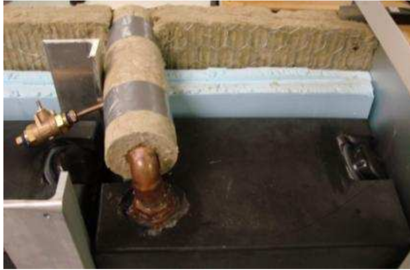
Figure 2.9 - Mineral Wool and Styrofoam Insulation used in the Unit
