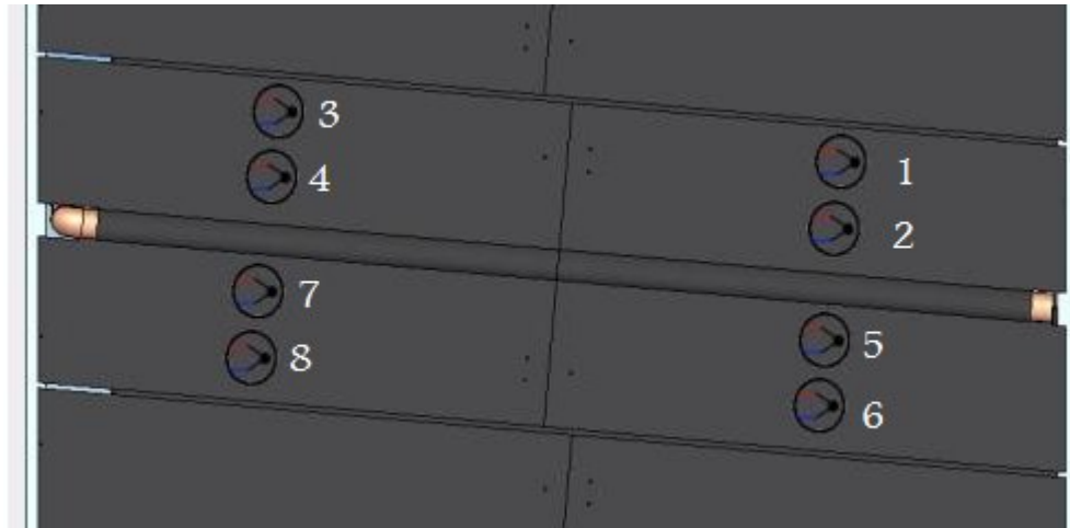
Figure IX.3 – Thermocouple Placement on the Absorber Plates
