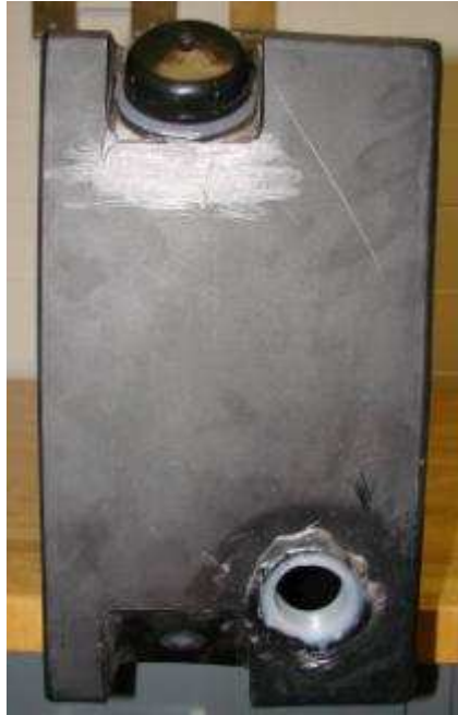
Figure 2.6 - Female Fitting and Fill-up Cap on the side of the Water Tank
