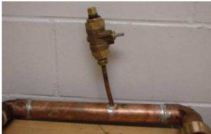
Figure 2.3 - Filling feature of the Heat Pipe.
