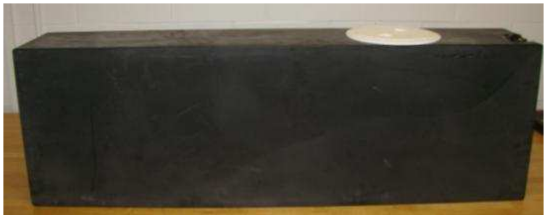
Figure 2.5 – Plastic Water Tank used for Thermal Mass
