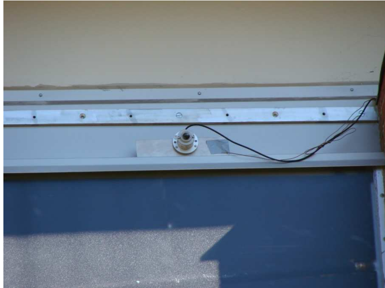
Figure 2.17 – Kipp & Zonen CM3 Pyranometer and Mounting
