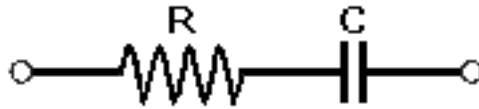
Figure 1. A schematic representation of the circuit model that Giaever and Keese (1991) used to represent the electrochemical system. R is a resistor, and C is a capacitor.
