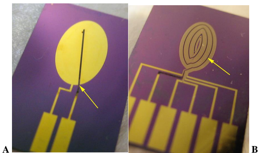
Figure 4.24 – Post processing photographs of the Ag|AgCl pseudo-electrodes for the two electrode (A) and six electrode (B) sensors. Arrow indicated pseudo reference
