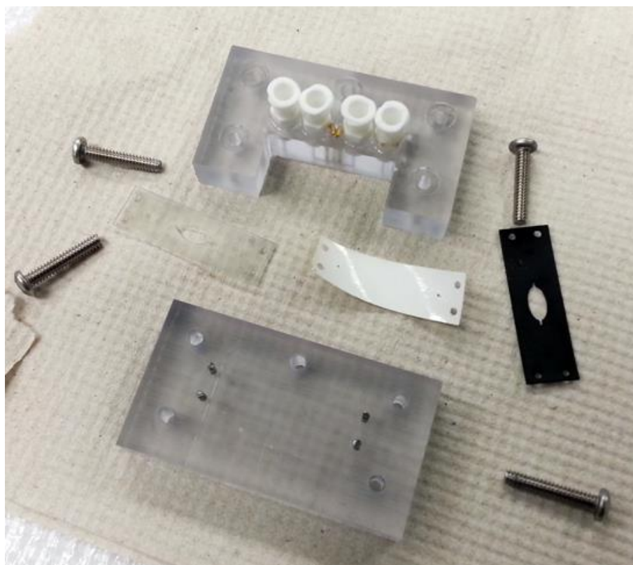
Figure 4.58 – View of all parts needed for assembly of the second generation flow cell.
