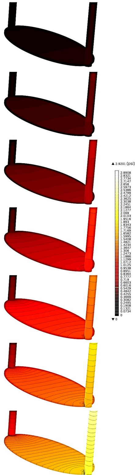
Figure 4.8 – CFD results for simulating the increase in pressure with increasing flow rate. Color scale indicates pressure magnitude. Black lines indicate equivalent lines of pressure in the volume.
