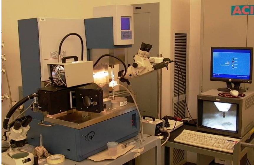
Figure 35. Overall test setup for insertion and retention force experiments in the eyes
