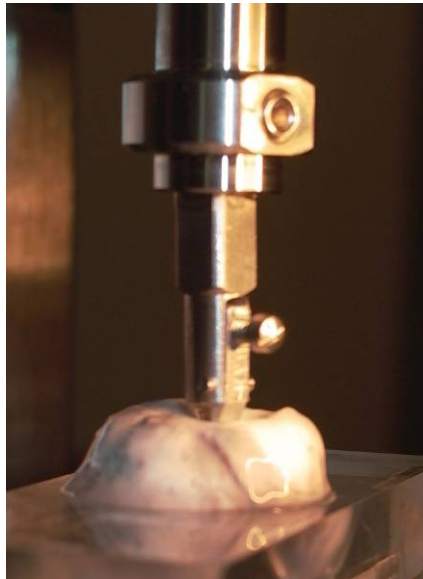
Figure 38. Insertion of microtack demonstrating tissue compliance issues
