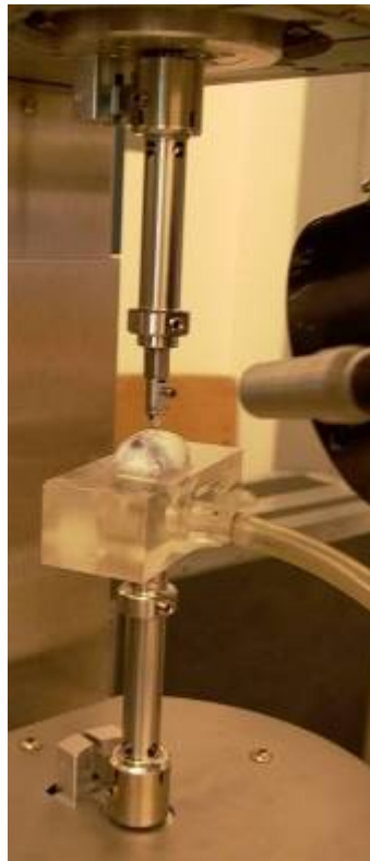
Figure 36. Close up of vacuum fixture holding a porcine eye
