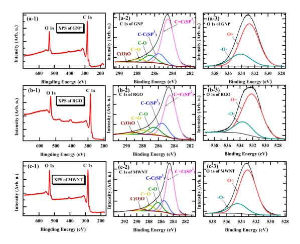
Figure 6.2 The XPS spectra of (a-1) GNP, (b-1) RGO, and (c-1) MWNT; C 1s binding energy of (a-2) GNP, (b-2) RGO, and (c-2) MWNT; O 1s binding energy of (a-3) GNP, (b-3) RGO, and (c-3) MWNT.
