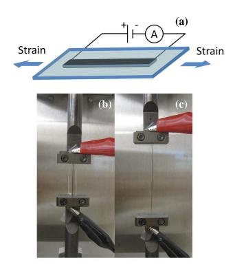
Figure 7.3 The test setup to measure the strain-resistance relationship of the strain sensor: (a) a schematic diagram of the test setup, strain is applied to the both ends of the sensor, and two-probe electrode connections are made at both ends of RGO film using copper wires; (b) the strain sensor free of strain; (c) strain sensor under 100% strain
