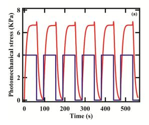
Figure 5.8 The photo-mechanical responses and the actuation stress response of binary mixture nano-carbons polymer composites actuator for 15% pre-strain.
