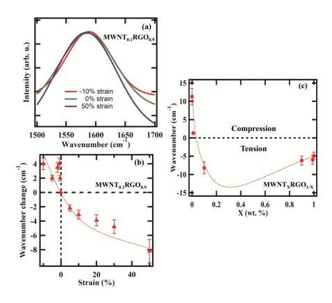
Figure 5.4 Load transfer (G-band) in  $RGO_{0.9}MWNT_{0.1}/PDMS$ : (a) the Raman intensity versus wavenumber; (b) the change of the Raman peak in wavenumber as a function of the strain; and (c) the Raman peak shift in wavenumber versus the relative weight fraction of nano-carbons under 50% uniaxial tension.
