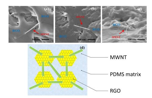
Figure 5.2 (a-c) The SEM images of  $MWNT_xRGO_{1-x}/PDMS$  matrix, and (d) the schematic representation of the RGO-MWNT/polymer system based on the above SEM images.
