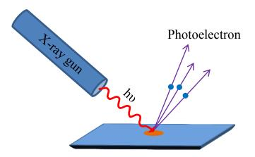
Figure 2.18 A schematic process image of the X-ray photoelectron spectroscopy
