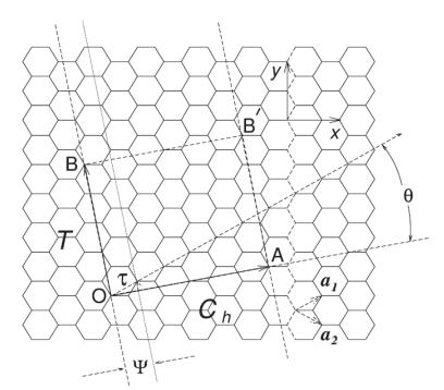
Figure 2.2 A geometrical view of the relationship between carbon nanotube and graphene [68].
