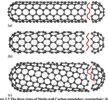
Figure 2.3 The three types of Single-wall Carbon nanotubes: (a)armchair; (b)zigzag; (c) chiral [48].
