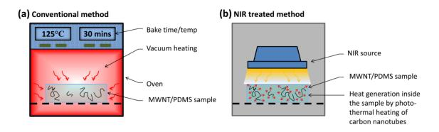
Figure 3.1 Schematic of the two different polymerization techniques: (a) oven based heating; (b) NIR light treatment.
