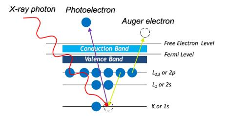
Figure 2.19 The schematic diagram of the photoelectric process (purple) and the Auger process (yellow).
