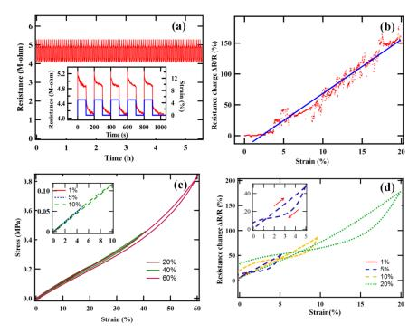
Figure 7.7 (a) The resistance of the strain sensor over time under 100 times cyclic loading of 5% tension strain, the inset is five times cyclic loading in detail; (b) resistance change versus strain of strain sensor; (c) the cyclic stress-strain curves of strain sensor; (d) the resistance change of the strain sensor under cyclic loadings of different maximum strain.
