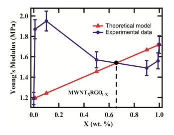
Figure 5.7 The Young's modulus versus weight percentage of nano-carbon filler for  $MWNT_{X}RGO_{1-X}/PDMS$  composite calculated using the rule of mixtures and compared to the experimental data.
