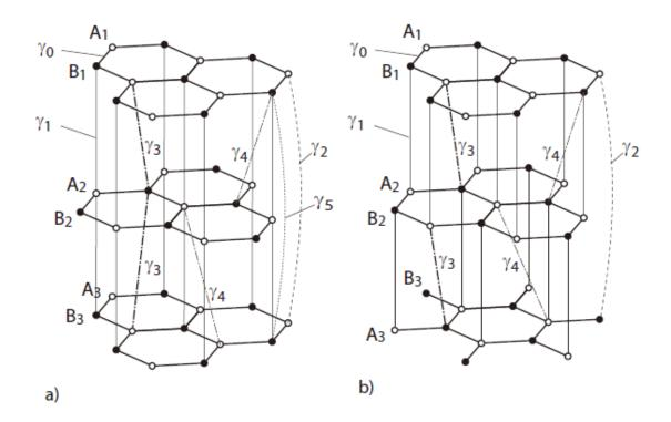
Figure 2.8 The crystal structure of (a) Bernal stacked and (b) Rhombohedra stacked few layer graphene with the complete set of tight binding parameters [81].
