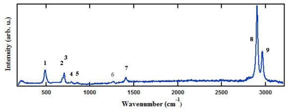
Figure 2.11 The Raman spectra of PDMS. The peaks labeled 1-9 are the different vibrational peaks of Si-O-Si and CH<sub>3</sub> groups.
