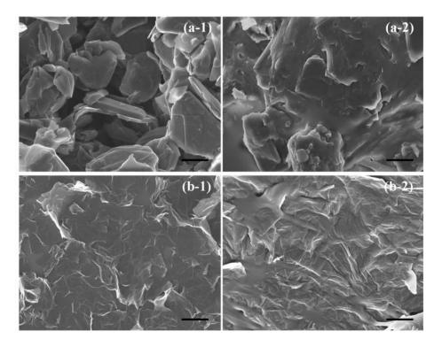
Figure 4.2 SEM images of (a-1) GNP; (a-2) GNP/PDMS; (b-1) RGO; (b-2) RGO/PDMS
