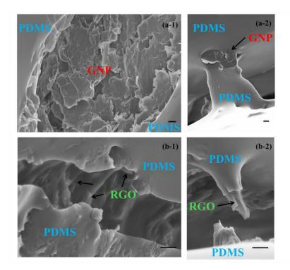
Figure 4.3 SEM images of the cracks (a-1) collapsed GNPs on the crater of the micro-crack; (a-2) GNPs aiding load transfer; (b-1) RGO between the crack openings; (b-2) cracking of RGO filler after peeling of PDMS. Scale bar: 500 nm in all the images.
