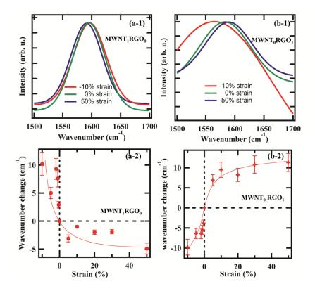
Figure 5.3 (a-1) & (b-1) plot the Raman intensity versus the shift in wavenumber under uniaxial tension and under uniaxial compression for  $MWNT_1RGO_0$  and  $MWNT_0RGO_1$ , respectively; (a-2) & (b-2) plot the change of the shift in wavenumber versus the strain under uniaxial tension and under uniaxial compression for  $MWNT_1RGO_0$  and  $MWNT_0RGO_1$ , respectively
