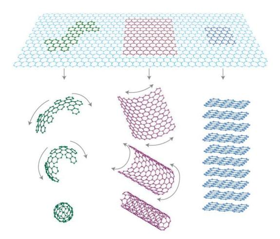
Figure 2.4 Mother of all graphitic forms. Graphene is a 2D building material of all other dimensionalities. It can be wrapped up into 0D fullerene, 1D carbon nanotube, and 3D graphite [58].
