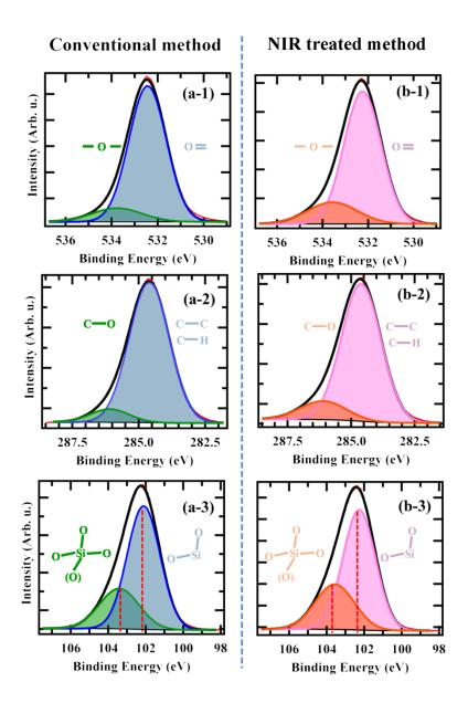
Figure 6.3 The XPS peaks of O1s, C1s, and Si2p measured for the MWNT/PDMS composites synthesized by (a) the conventional baking method and (b) NIR photon-assisted polymerization.
