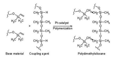
Figure 2.10 Schematics of PDMS polymerization based on PDMS oligomers and crosslinker [111]
