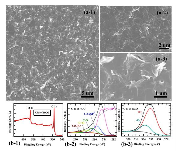
Figure 7.4 (a) The SEM images of the RGO film under different magnifications; (b-1) the XPS spectrum of the RGO film; (b-2) the C1s and (b-3) the O1s peaks with multiple-component simulation.
