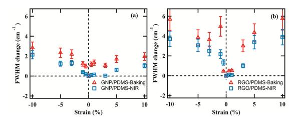
Figure 4.6 G-band FWHM value of GNP/PDMS (a) and RGO/PDMS (b) polymerized by conventional baking (blue) and NIR photon-assisted method (red) versus strain
