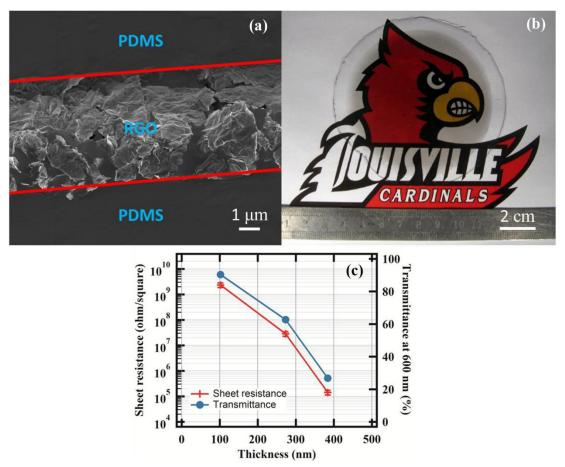
Figure 7.6 (a) The SEM cross-section image of the sandwich-structured strain sensor; (b) the large diameter ~ 10 cm sandwiched structure laminar composites; (c) the sheet resistance and the transmittance at 600 nm of different thickness.
