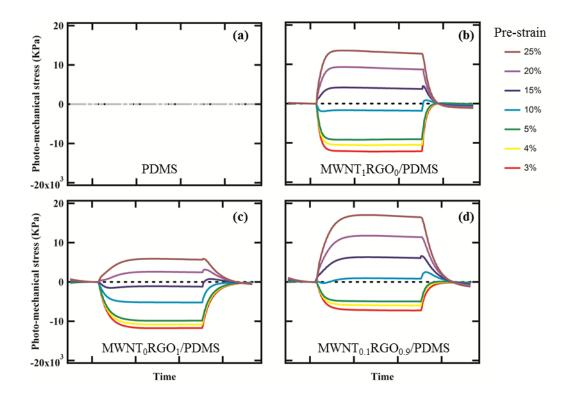
Figure 5.10 The comparison of increasing photomechanically induced stress change in binary mixture nano-carbons polymer composites actuator as a result of NIR illumination: (a) plain PDMS; (b) MWNT<sub>1</sub>RGO<sub>0</sub>/PDMS; (c) MWNT<sub>0</sub>RGO<sub>1</sub>/PDMS; (d) MWNT<sub>0.1</sub>RGO<sub>0.9</sub>/PDMS.
