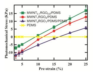
Figure 5.11 The average photomechanically response versus the pre-strain of binary mixture nano-carbons polymer composites actuator with different weight ratio
