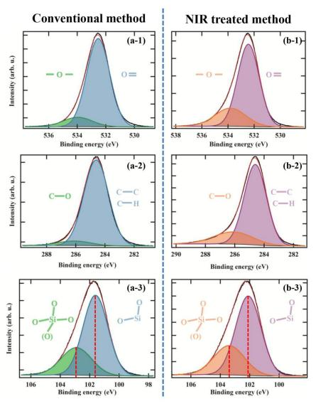
Figure 6.4 The XPS peaks of O1s, C1s, and Si2p measured for the RGO/PDMS composites synthesized by (a) the conventional baking method and (b) NIR photon-assisted polymerization.
