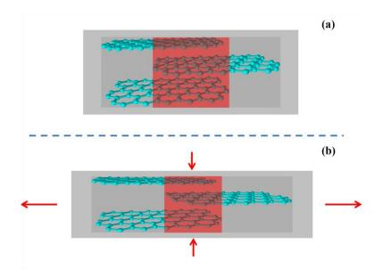
Figure 7.8 The mechanism of PDMS/RGO/PDMS sandwiched structure strain sensor: (a) the strain sensor free of strain; (b) the strain sensor under the tensile strain.
