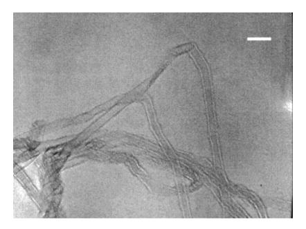
Figure 2.1 The TEM image of carbon nanotubes [63]. Scale bar: 20 nm.
