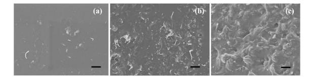
Figure 3.2 SEM images of the MWNT/PDMS samples, scale bar 500 nm; (a) 0.01 wt. %; (b) 0.1 wt. %; (c) 1 wt. % of MWNT.
