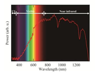
Figure 6.1 The spectrum profile of halogen lamp with UV filter
