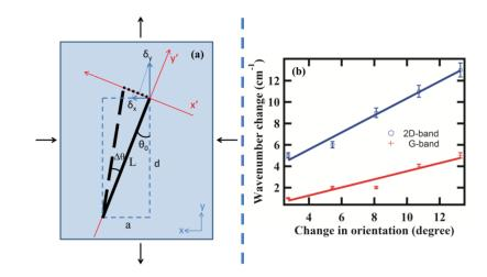
Figure 5.5 (a) Model describing the change in orientation of the nanotube in polymer on application of a uniaxial tensile strain, (b) the change in Raman
