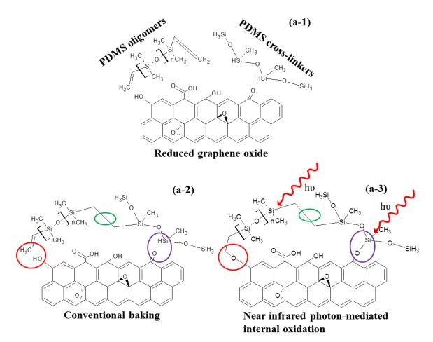
Figure 6.5 (a-1) The chemical structures of the PDMS oligomer and the PDMS cross-linker; (a-2) the reaction model of the conventional baking polymerization; (a-3) the reaction model of the NIR photon-assisted polymerization.
