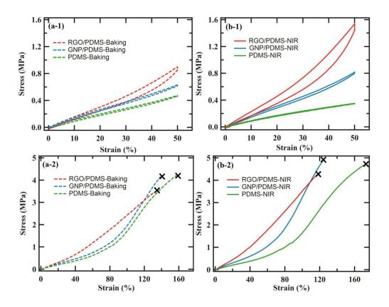
Figure 4.7 Cyclic stress-strain curves (a-1) and stress-strain curves (a-2) until failure of pure PDMS, RGO/PDMS, and GNP/PDMS polymerized by conventional baking method; Cyclic stress-strain curves (b-1) and stress-strain curves (b-2) until failure of pure PDMS, RGO/PDMS, and GNP/PDMS polymerized by NIR photon-assisted method.
