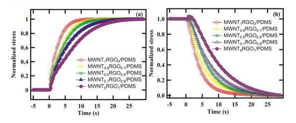
Figure 5.9 (a) Actuation and (b) relaxation of the binary mixutre nano-carbons polymer composites actuator
