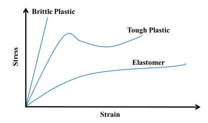
Figure 2.9 The Stress-strain behavior of various polymers [108]
