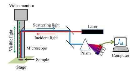
Figure 2.12 The schematic of a Raman spectrometer
