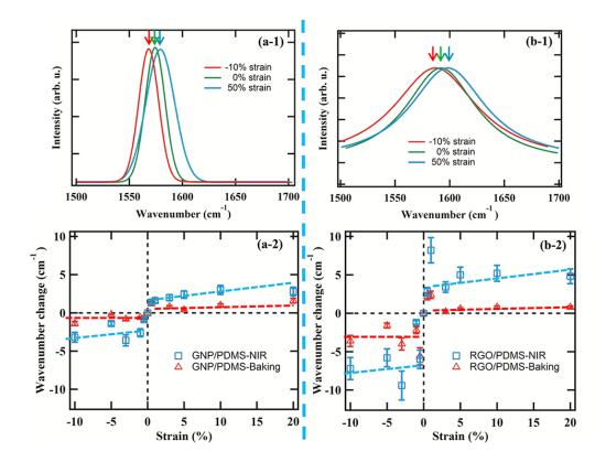
Figure 4.5 Load transfer: G band shift in (a-1) GNP/PDMS and (b-1) G band shift; change in wavenumbers with strains of (a-2) GNP/PDMS and (b-2) RGO/PDMS.
