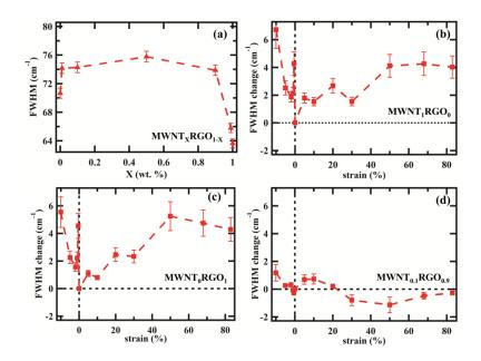
Figure 5.6 The Full Width Half Maximum (FWHM) data for the different compositions of MWNT<sub>x</sub>RGO<sub>1-x</sub>/PDMS: (a) the FWHM versus weight fraction of the nano-carbon; (b) the FWHM change versus percentage strain for MWNT<sub>1</sub>RGO<sub>0</sub>/PDMS; (c) the FWHM change versus strain for MWNT<sub>0</sub>RGO<sub>1</sub>/PDMS; and (d) the FWHM change versus strain for MWNT<sub>0.1</sub>RGO<sub>0.9</sub>/PDMS.
