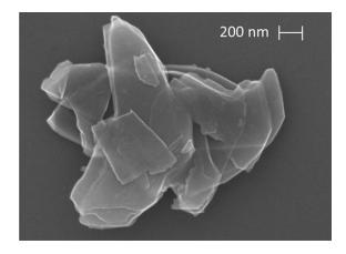
Figure 2.7 The SEM images of graphene nanoplatelet [79].
