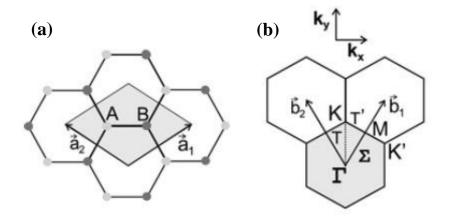
Figure 2.16 (a) The shadowed area is a real-space unit cell of graphene showing the inequivalent atoms A and B and unit the vectors  $a_1$  and  $a_2$ ; (b) the shadowed area is a reciprocal-space unit cell showing the 1<sup>st</sup> Brillouin zone [151].
