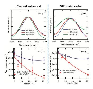
Figure 3.4 Load transfer in the conventional (a-1) and NIR light polymerized samples (b-1); the change in the wavenumber is displayed as a function of the percentage strain for the conventional (a-2) and NIR light polymerized samples (b-2).
