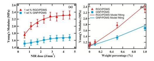
Figure 4.8 (a) Young's modulus versus NIR light dose for RGO/PDMS (red line) and GNP/PDMS (blue line) fractions; (b) change in Young's modulus versus weight percentage of RGO (red line) and GNP (blue line) for NIR light treated.
