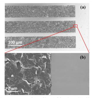
Figure 7.5 (a) The clear pattern of the ~  $80\mu m$  RGO stripes with ~ $20 \mu m$  spacing; (b) the sharp pattern edge formed by etching.
