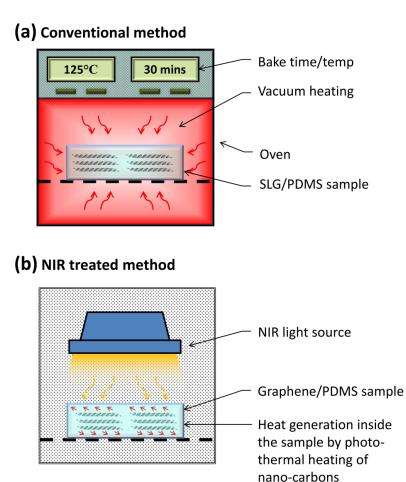
Figure 4.1 Schematic of the two different polymerization techniques: (a) oven based heating; (b) NIR light treatment method.
