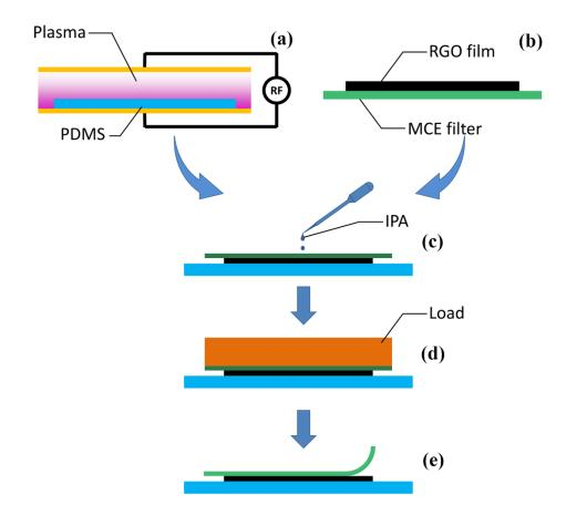
Figure 7.1 The schematic of the RGO film transfer process
