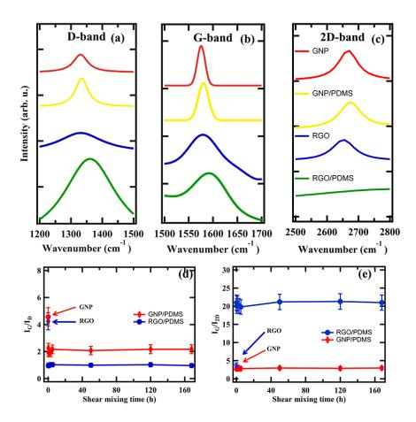
Figure 4.4 Raman spectra of (a) D band, (b) G band, (c) 2D band of GNP, RGO, GNP/PDMS, and RGO/PDMS, (d) and (e) ratio of  $I_G/I_D$  and  $I_G/I_{2D}$  versus shear mixing time respectively
