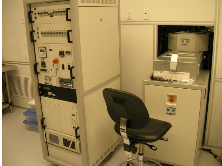
Figure 2-3. STS DRIE machine at the University of Louisville.
