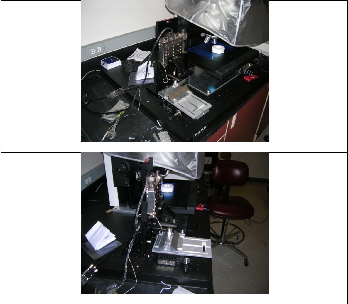
Figure 2-19. Actuator, load cell, and bending structure.
