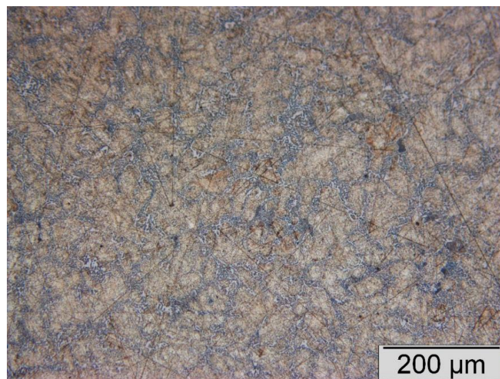
Figure A.20: Optical microscopy imaging of etched FFF 3D cast Sn60Bi40 sample (5X, Bright field)
