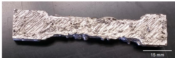
Figure 3.6: FFF 3D printed ASTM E8 standard tensile specimen of Sn60Bi40 alloy
