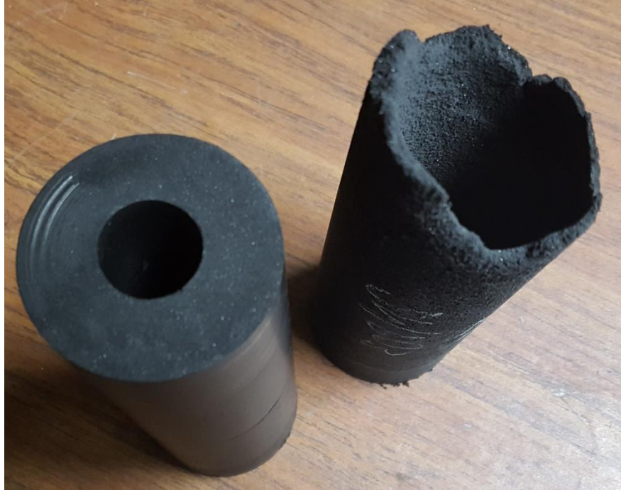
Figure 8 - Examples of a fully-formed carbon block, left, and a block that was not sufficiently heated and formed, right.
