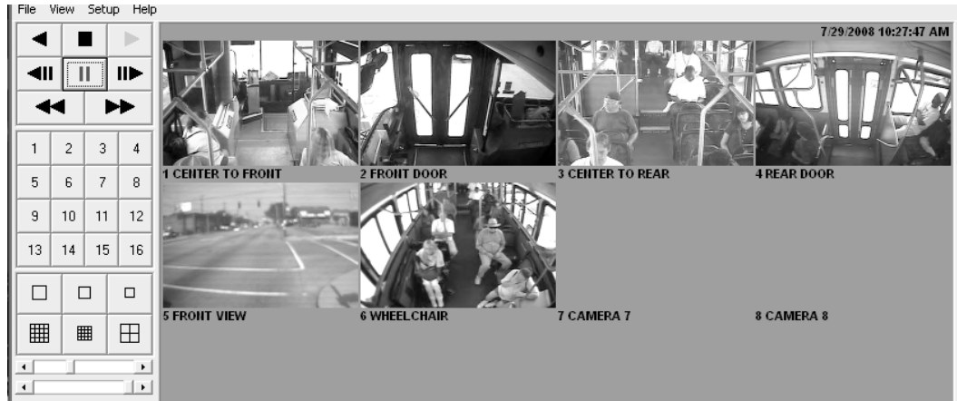
Figure 1. In-vehicle 6-camera LATV video surveillance system. This LATV was equipped with cameras to include views from the front windshield, front and rear of the LATV interior, and front and rear doors, as well as the wheelchair securement station.
