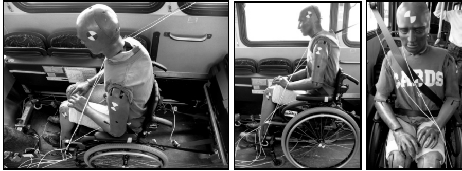
Figure 2A. Typical test setup of 50 th percentile ATD seated in manual wheelchair with four tie-downs and lap and shoulder belt applied. Low-g accelerometers were mounted in the ATD head, chest, and pelvis as well as the LATV floor (at securement station) while load cells were used to measure webbing tension in the tie-downs and lap and shoulder belts.
