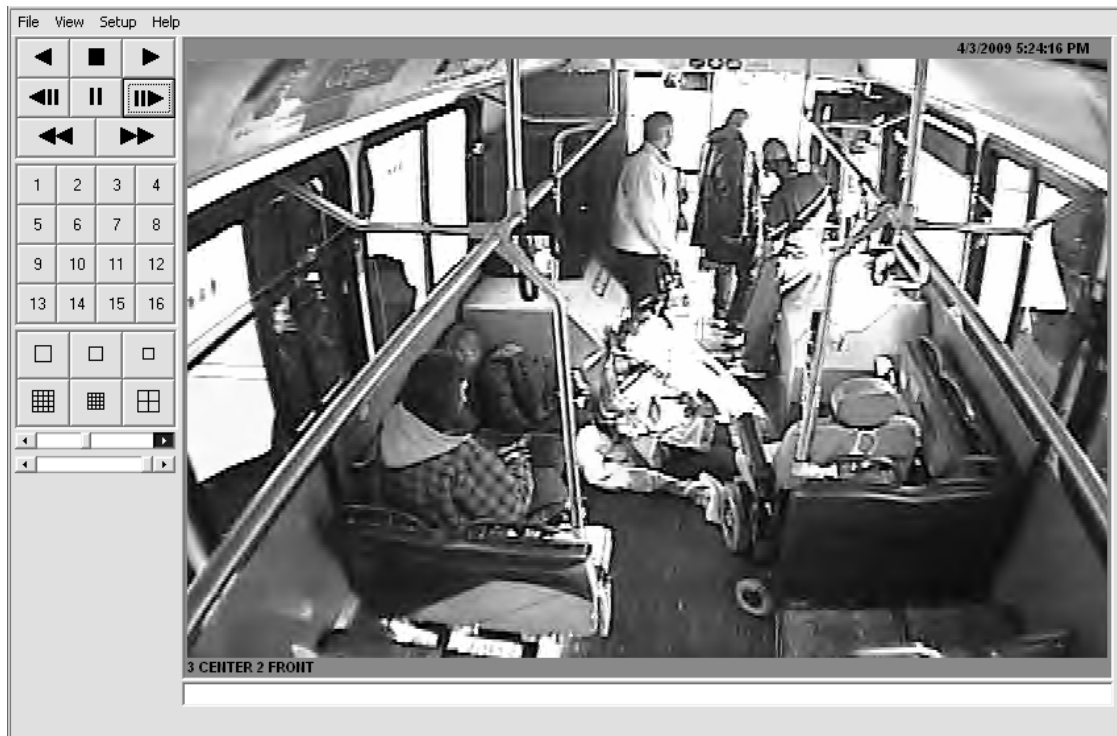
Figure 8. Case 3: Power wheelchair passenger ejected from wheelchair during normal LATV braking. Wheelchair passenger struck the bulkhead in front of the securement station and fell to the floor complaining of a fractured leg. (View from LATV rear).
