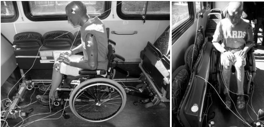
Figure 1A. Test setup of 50 th percentile ATD seated in manual wheelchair within LATV securement station. The lap belt was used in an attempt to secure the wheelchair (routed around the seatback). The tiedowns and shoulder belt were not applied.
