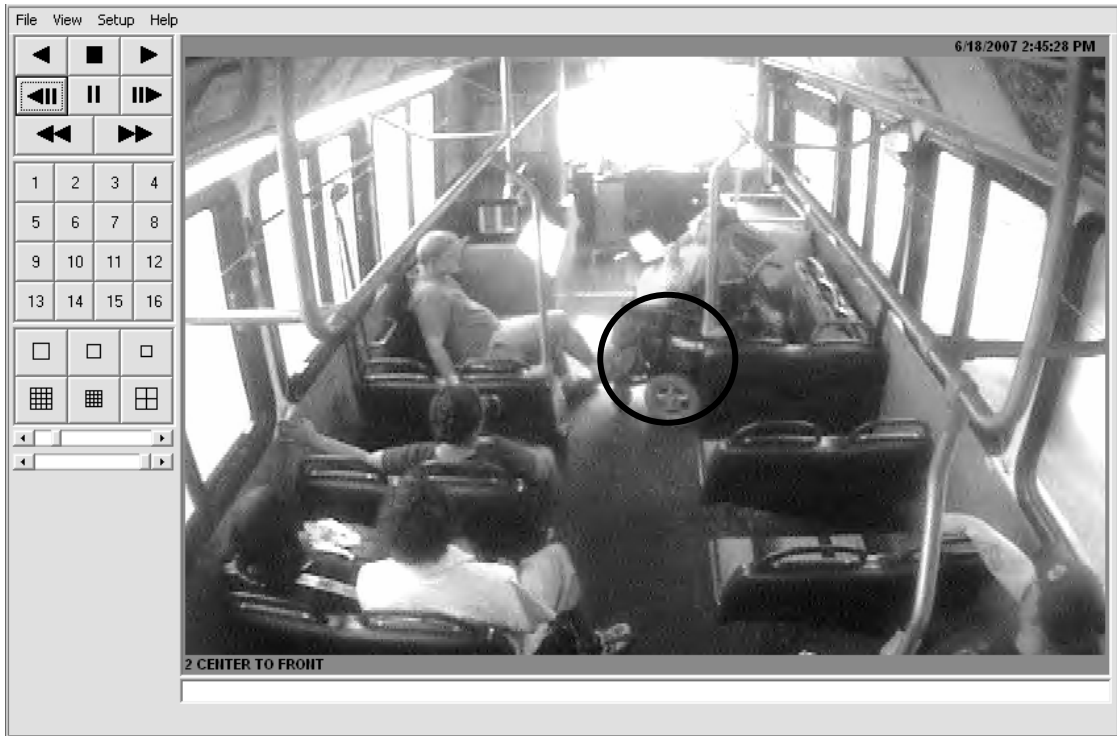
Figure 4. Case 1: Unsecured power wheelchair enters aisle during routine LATV transit, while sitting ambulatory passenger lifts foot to prevent injury and limit power wheelchair movement. (View from LATV rear).
