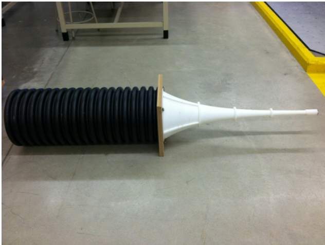
Figure 20 Anechoic termination prototype with catenoidal horn (white) and absorbing termination (black) of length 0.91 m (36 in.) and diameter 0.305 m (12 in.)
