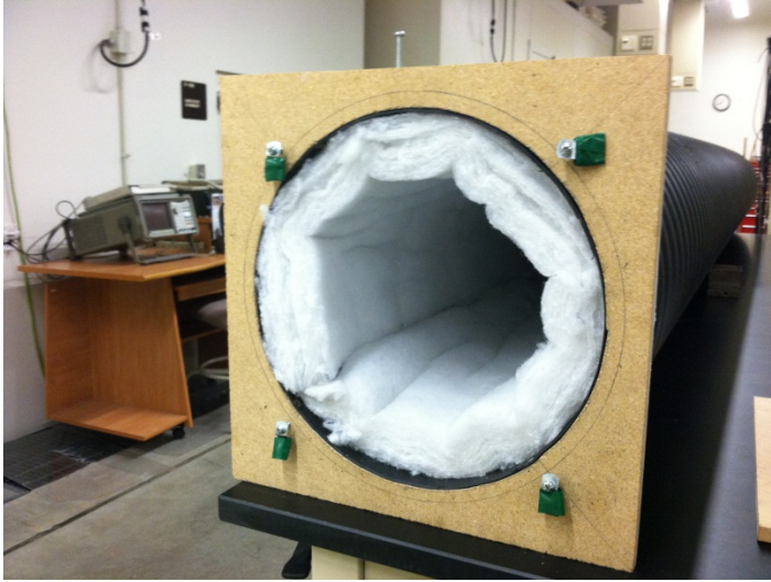
Figure 22 Inlet of the absorbing termination with the horn unattached to the medium density fiberboard. A layer of polyester fiber lines the circumference throughout the termination
