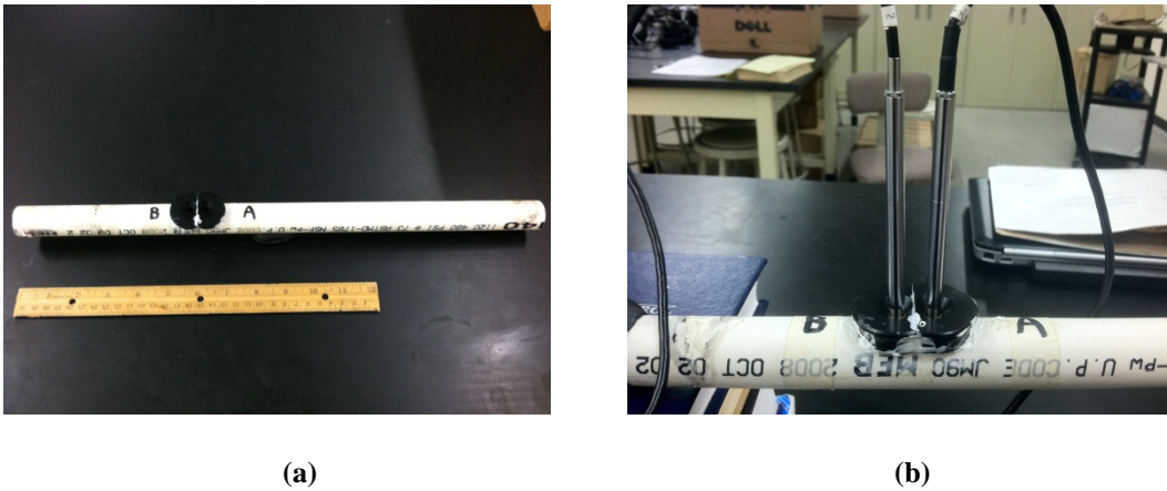
Figure 28 Impedance tube (left) and close-up of microphone mounts (right)
