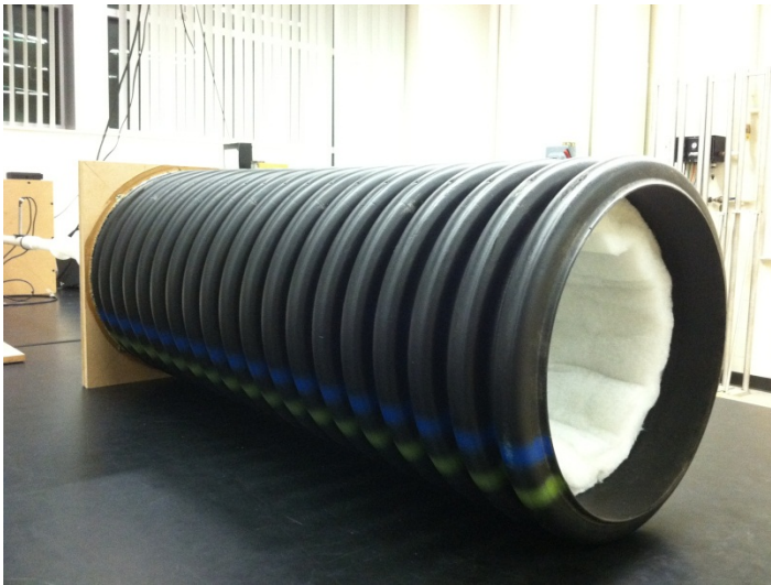
Figure 24 Absorbing termination with open end. Horn is partially visible on the far left
