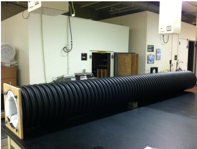
Figure 21 An absorbing termination 3.28 m (129 in.) in length and diameter 0.305 m (12 in.). The mouth of the horn connects to the end shown on the left
