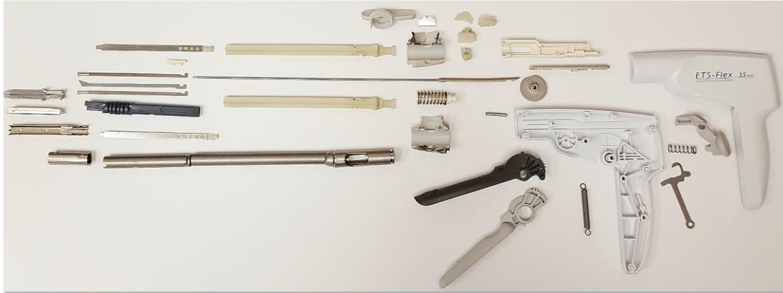
Figure 19. Ethicon Endo-Surgery Endopath® ETS Endoscopic Articulating Linear Cutter exploded view.
