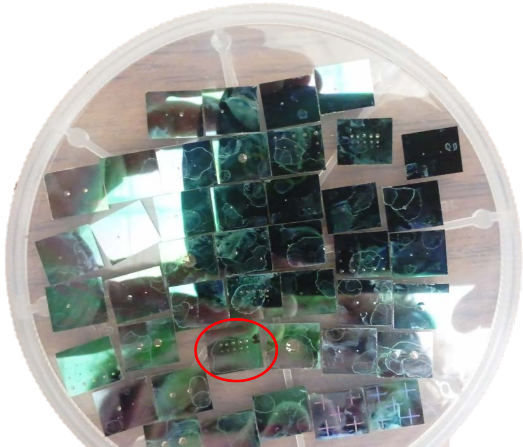
Figure 25. Released dies after manufacture – array 1 highlighted.
