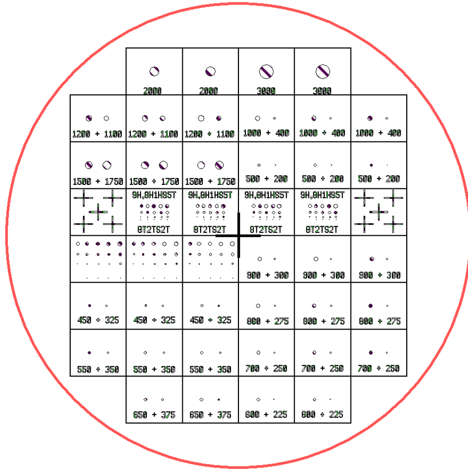
Figure 11. L-Edit mask layout for the 100mm diameter wafer.
