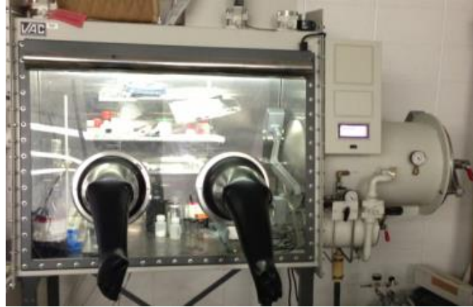
Figure 3.2. Argon filled glove box used for coin cell assembly
