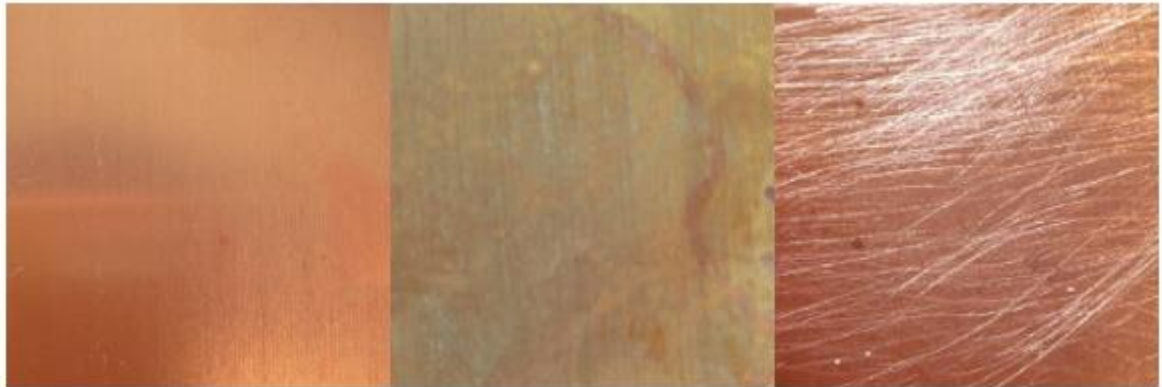
Figure 4.1. Copper surface images under different treatment (left: untreated, middle: chemical treated, and right: mechanical treated)
