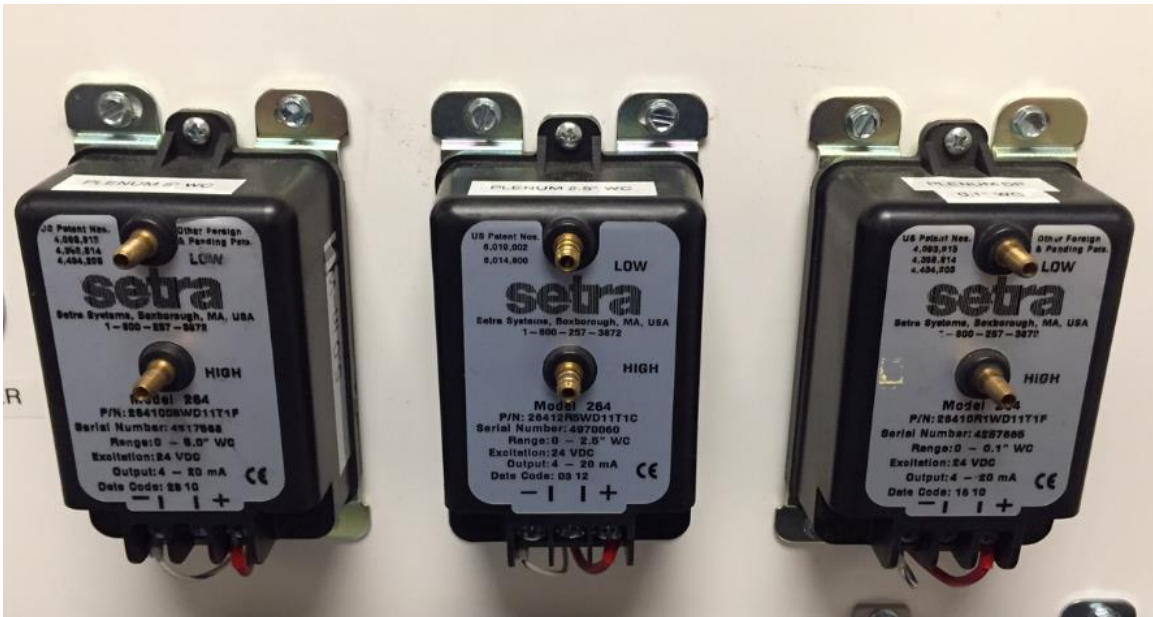
Figure 4.4: Setra Systems© differential pressure transducers used to measure pressure drop on the wind tunnel with ranges of 0-5” WC, 0-2.5” WC and 0-0.1” WC
