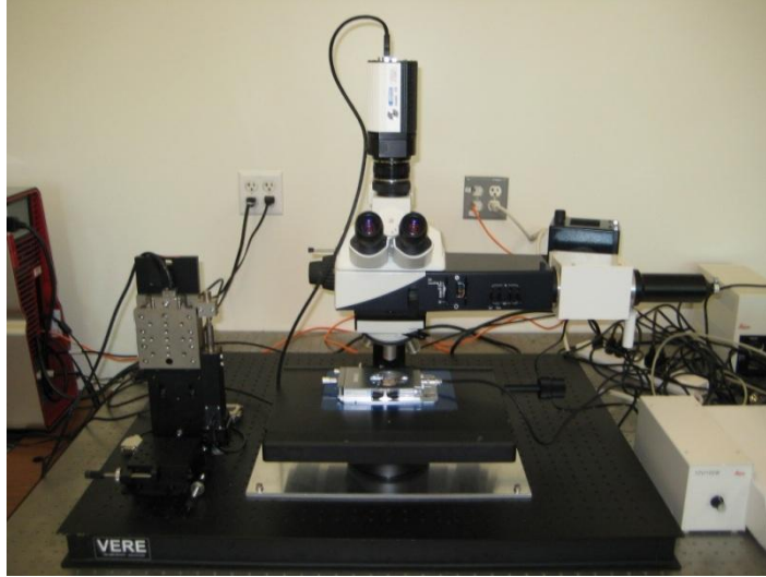
Figure 18. Leica MST49 optical microscope with Retiga-4000R.
