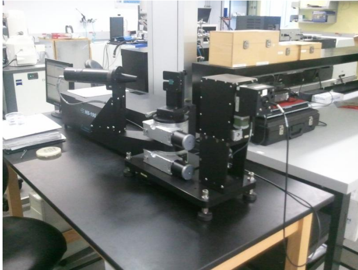
Figure 27. J.A Woollam WVASE32 ellipsometer.
