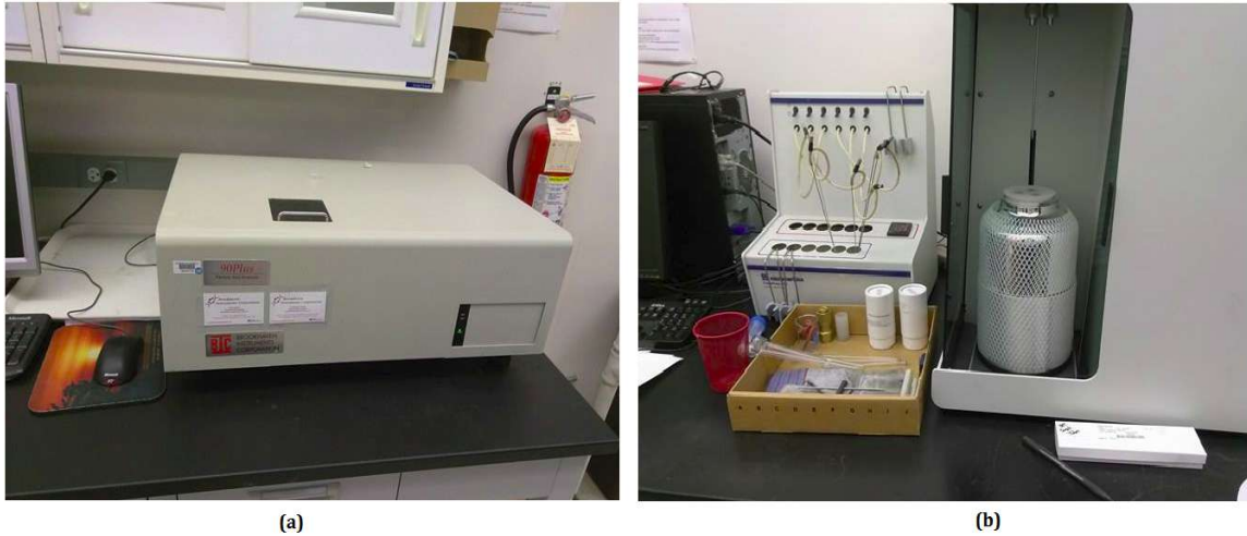
Figure 14. (a) Brookhaven 90Plus™ Particle size analyzer and (b) Micrometrics TriStar™ Surface Area and Porosity Analyzer
