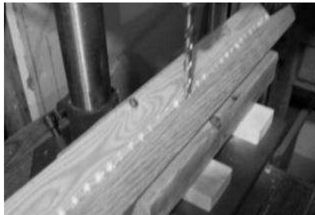
FIGURE 79 – Centering the Construction Jig on the Drill Press.
