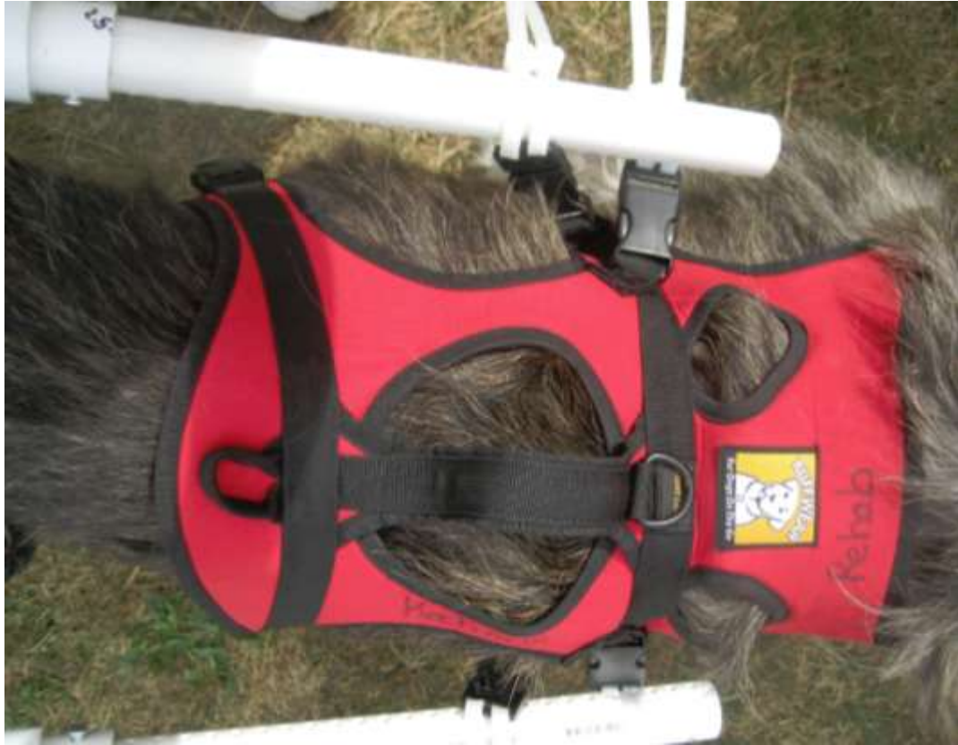
FIGURE 140 – Top View of the Chest Harness Attached to the Front of the Wheelchair.
