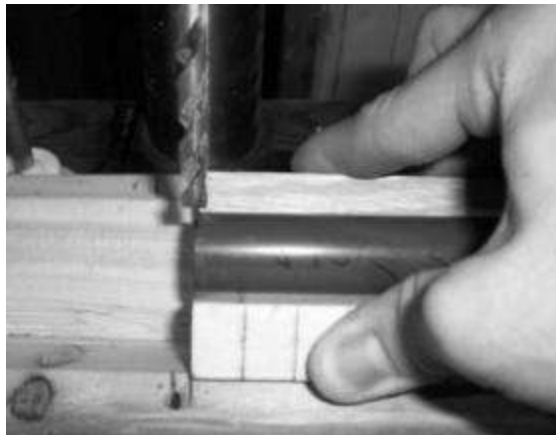
FIGURE 81 – Marking the “Zero” Line on the Base.
