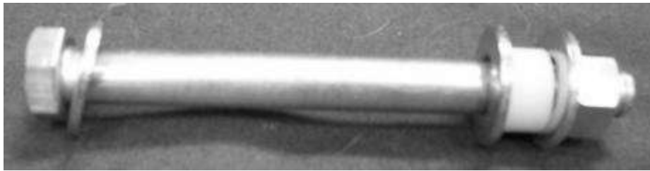
FIGURE 132 - Axle Assembly for Attaching the Wheels.
