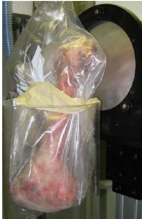
Figure 13. The pig femur specimen #2 placed in the digital X-ray scanner against the intensifier.
