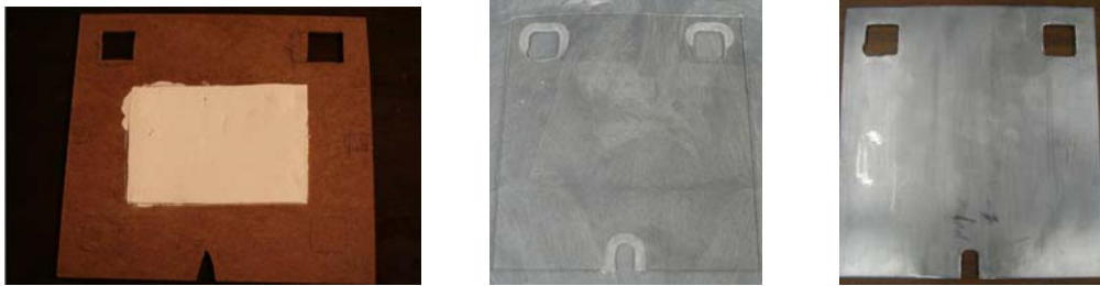
Figure 7. Plaster in a wooden cutout, a plexiglass and aluminum sheet to be placed on the intensifier.
