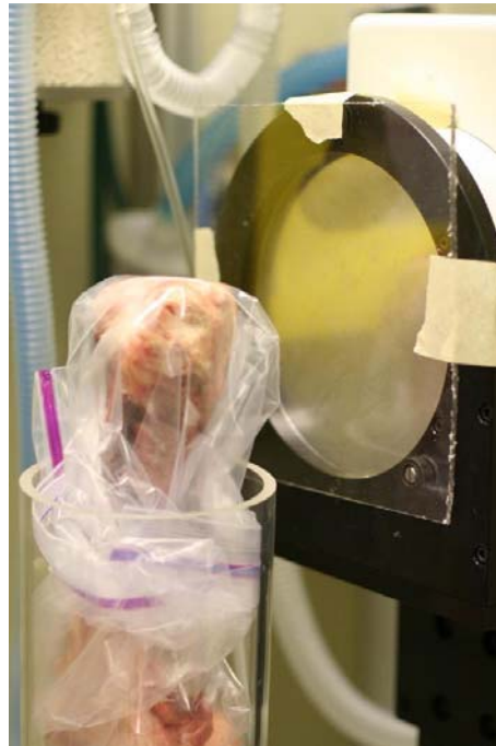
Figure 9. Pig femur specimen #1 in a plastic bag with a sheet of plexiglass placed on the intensifier.
