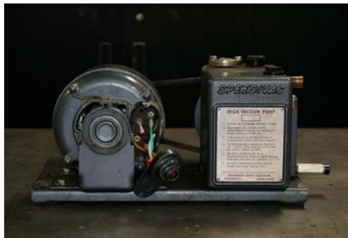
FIGURE 2.13 - Speedivac Vacuum Used To Charge The Heat Pipe.
