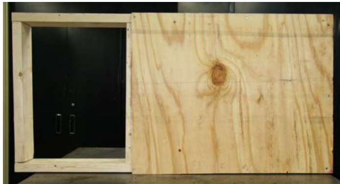
FIGURE 2.5 - Wall Construction For Experimental Model.
