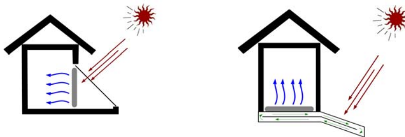
FIGURE 1.3 - Greenhouse and Isolated Gain Passive Solar Systems.
