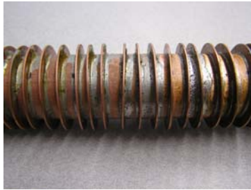
FIGURE 2.8 - Finned Condenser Section.
