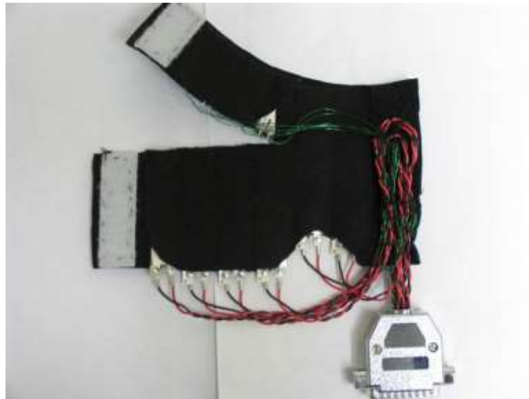
Figure 9: Prototype matrix using piezo-film sensors showing the placement of the sensor matrix.
