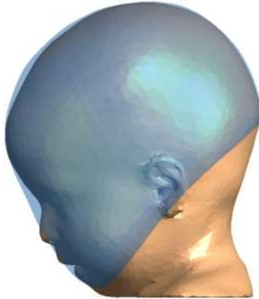
Figure 22: Lateral comparative overlay of 11-month-old child (3D reconstruction of CT imaging) and 12-month-old CRABI ATD (transparent; blue) highlighting morphological differences in head profile.
