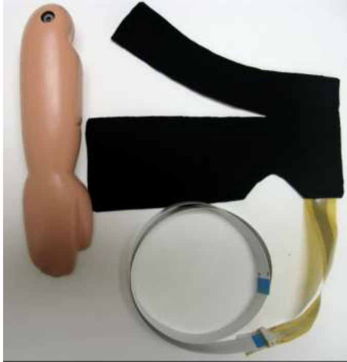
Figure 13: The forearm sensor matrix enveloped in neoprene, ready to be adapted to the ATD.
