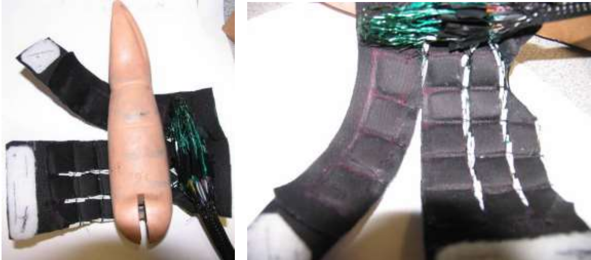
Figure 7: Prototype sensor matrix showing the placement of the sensors in relation to the forearm and associated wiring.
