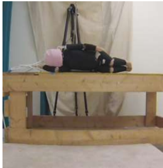
Figure 23: CRABI anthropomorphic test device (ATD) in side-lying, facing forward initial position for bed fall experiments. The pendulum actuator providing the initial force to the posterior torso of the ATD is located behind the ATD.
