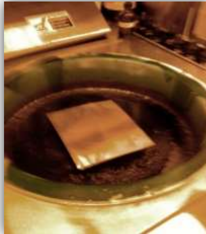
Figure C2: Copper substrate positioned within rotating machine tub after application of the photoresist.
