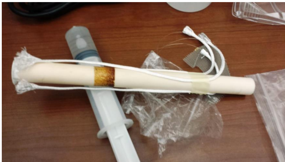
Figure 4.3: Alumina tube used for button cell testing with wires for current collection running along the outside and the button cell at one end.
