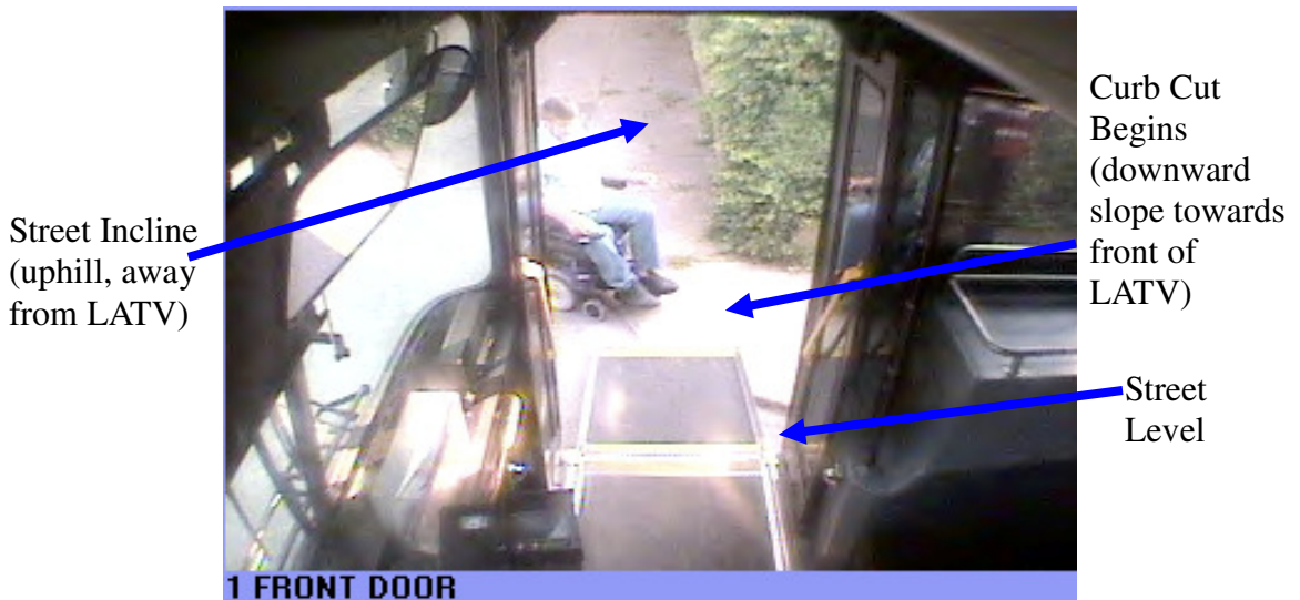
FIGURE 11 – Example of ramp deployment onto uneven surfaces
