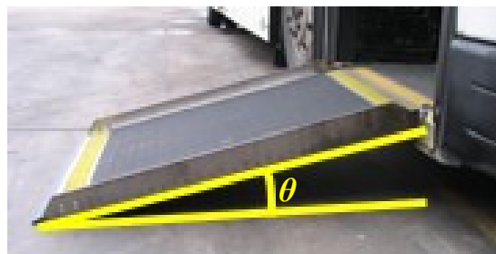
\theta indicates measured LATV ramp angle
