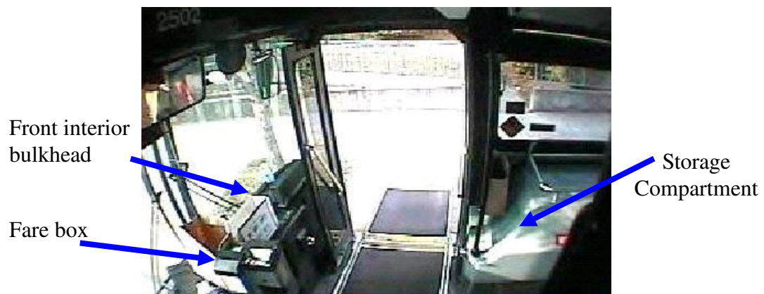
FIGURE 10 – Interior TARC LATV Components in Access Path
