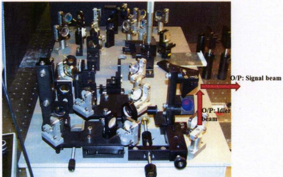
Figure 3.18 Optical alignment set up for Signal and Idler output
