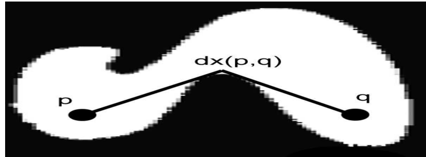
Figure 3.10: Example of a geodesic distance calculation between two points ( p and q ) on the boundary of a 2D MRI scan [98]. The area has been zoomed and binarized so that the curvature can be clearly seen.
