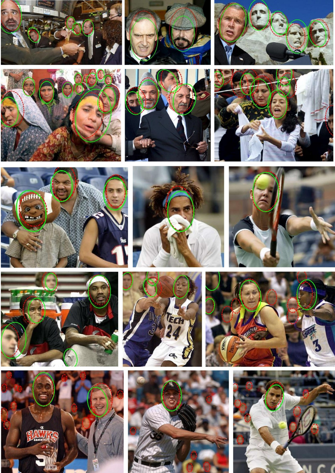
Figure 5.2: Examples of FDDB results showing detections as green ellipses and annotation as red dashed ellipses. The last row shows examples of the completely blurred faces annotated in this database.
